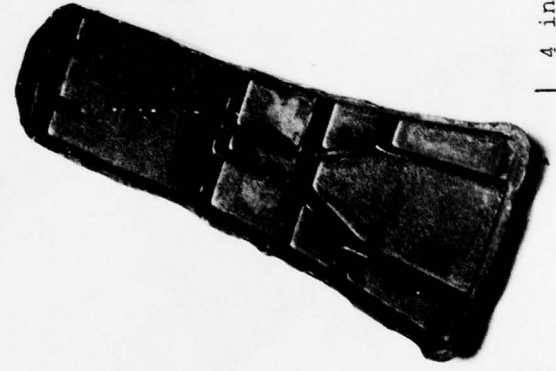
Figure 23 Closeup view of structural component forgings produced by isothermal forging at 1400F using three different lubricants
