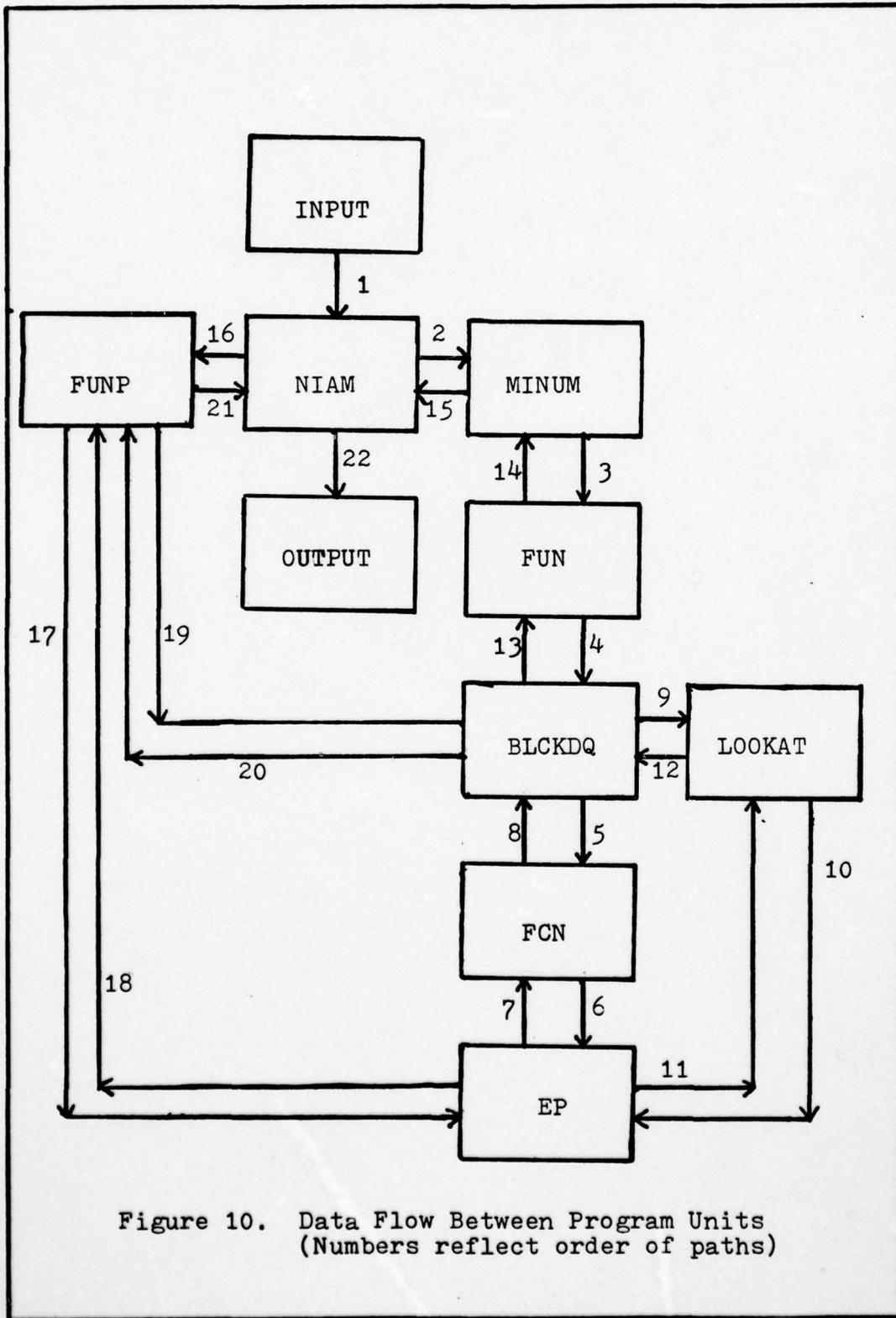
Figure 10. Data Flow Between Program Units
