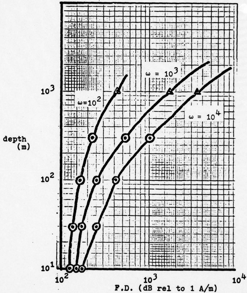
Figure 9. Depth variation of horizontal magnetic field density of atmospheric noise spectra with frequency. Circles are taken from Figure 2 (Ref 23:644), and triangles from Ref 3:328. Shows the corroboration of the two sources.
