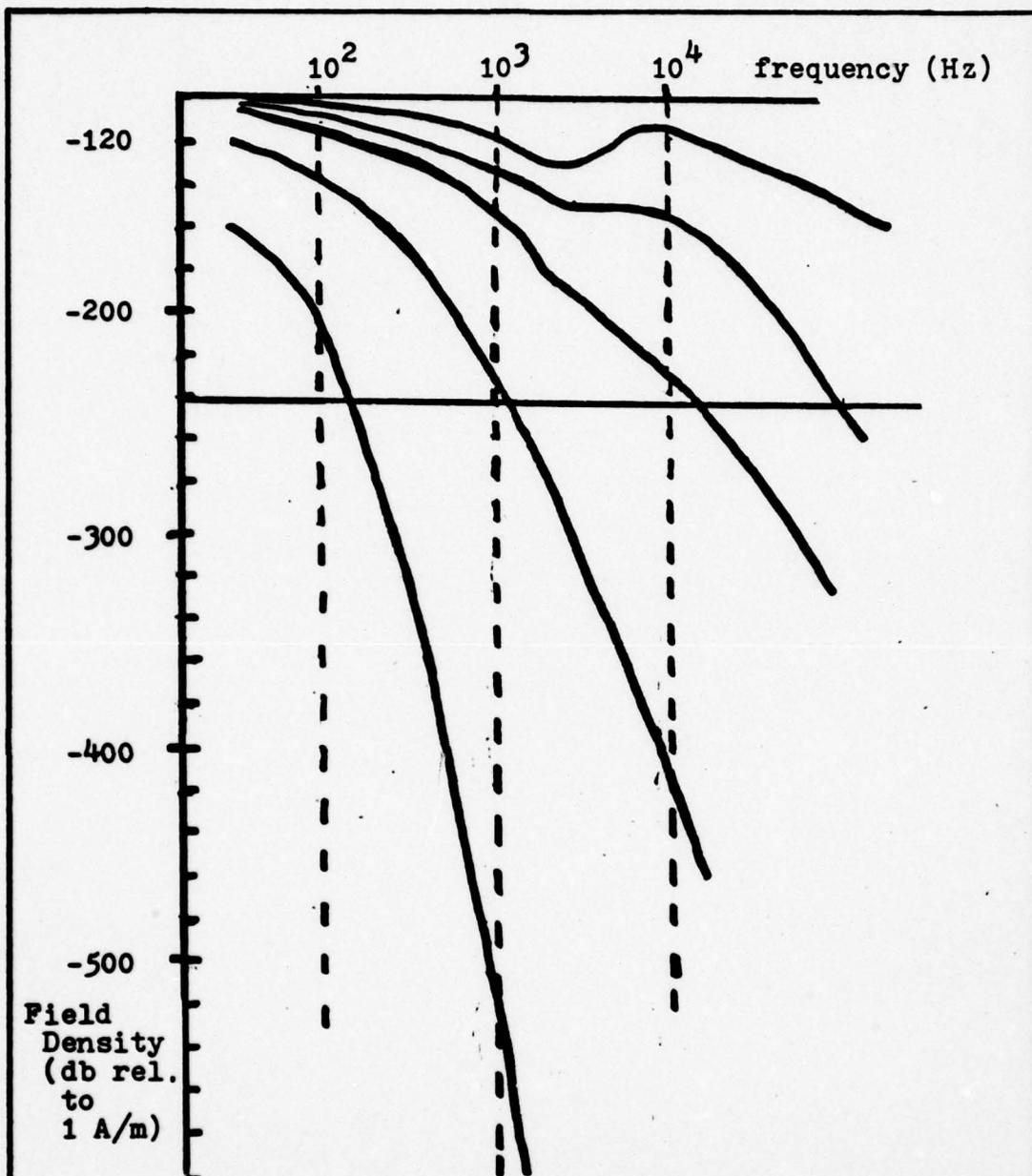
Figure 8. Frequency variation of horizontal magnetic field density of atmospheric noise spectra with oceanic depth (conductivity assumed to be 4 mho/m) (Ref 23:644).
