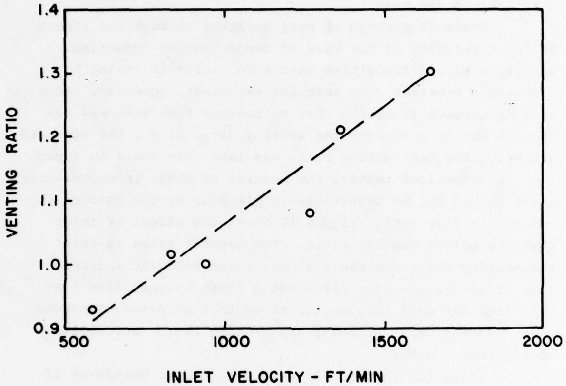
FIGURE 10. EFFECT OF INLET VELOCITY ON VENTING RATIO.
