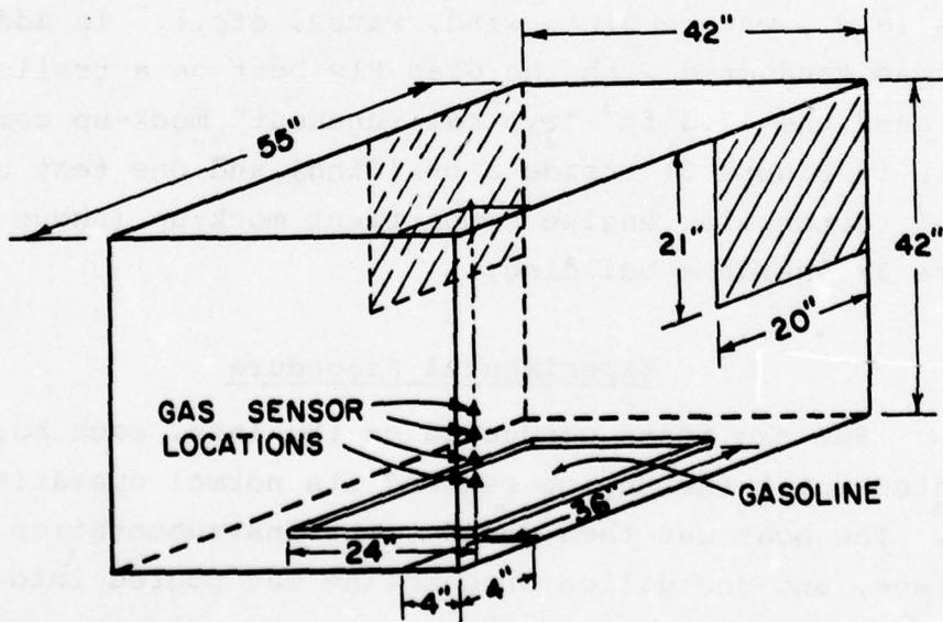
FIGURE 3. CONFIGURATION OF TYPICAL RUNABOUT (TOP) AND 56 FT<sup>3</sup> RECTANGULAR (BOTTOM) ENGINE COMPARTMENT MOCK-UPS.
