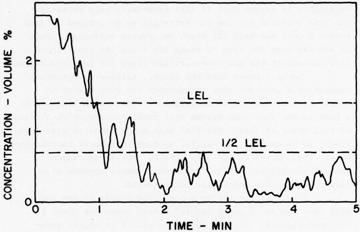
FIGURE 13. GASOLINE VAPOR CONCENTRATION AT THE GAS SENSOR LOCATED 1 INCH ABOVE THE FLOOR OF THE COMPARTMENT DURING TEST 5A (LIQUID FUEL).
