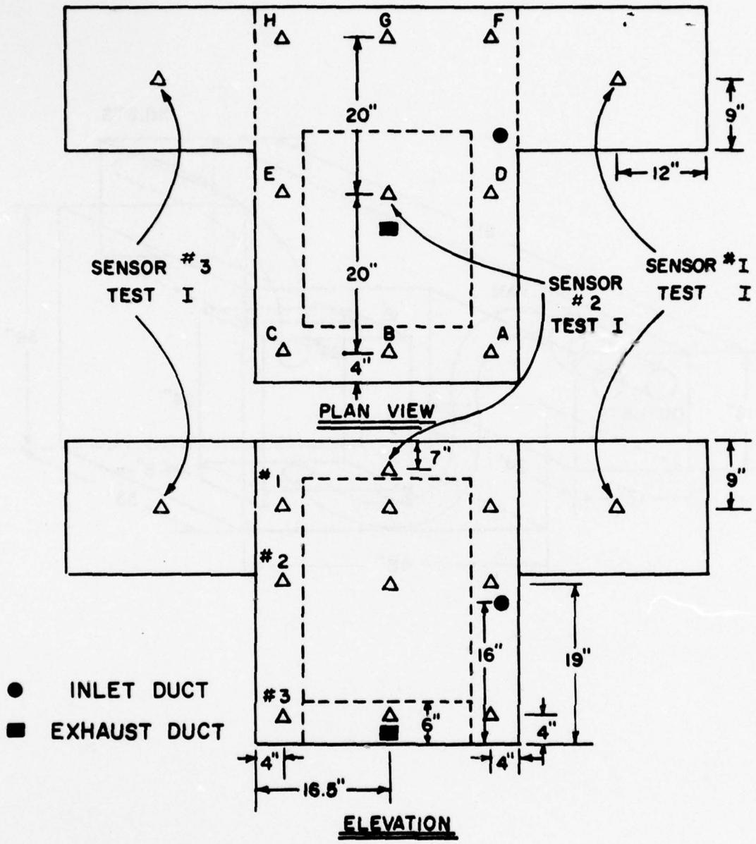
FIGURE 6. TYPICAL RUNABOUT ENGINE COMPARTMENT MOCK-UP SHOWING GAS SENSOR LOCATIONS AND DUCT TERMINATIONS FOR EACH TEST.
