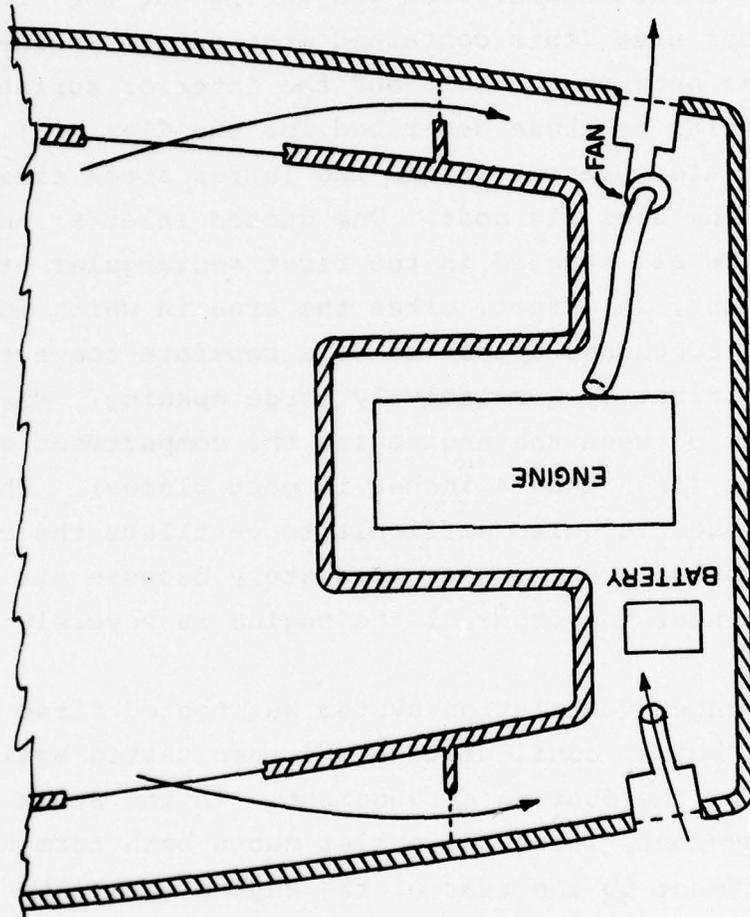
FIGURE 22. GENERAL LAYOUT OF RANGER ENGINE COMPARTMENT.
