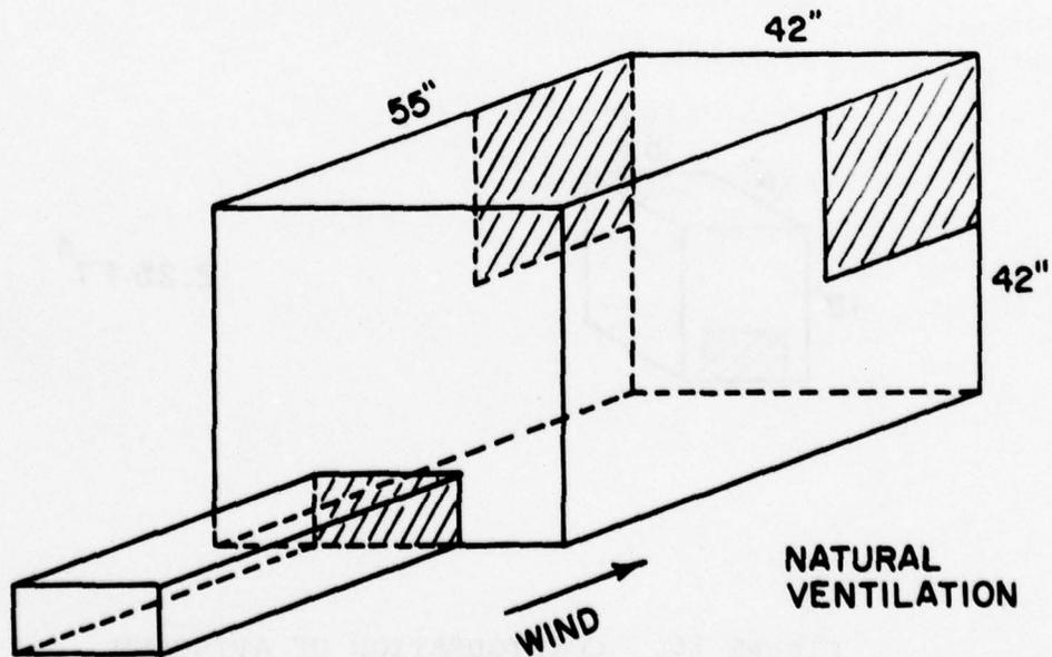
FIGURE 19. POSITION OF ATTACHED COMPARTMENTS DURING VENTING TESTS.
