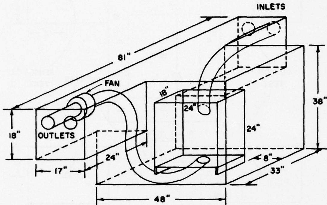
FIGURE 5. DIMENSIONS OF THE "TYPICAL RUNABOUT" COMPARTMENT.
