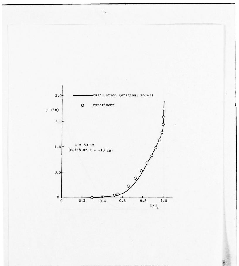
COMPARISON WITH THE DATA OF SCHUBAUER AND SPANGENBERG (VELOCITY PROFILE)
