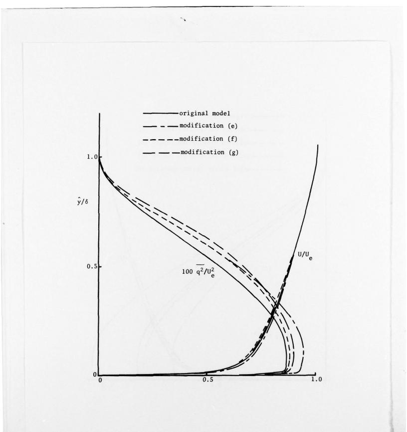
EFFECT OF MODIFICATIONS TO THE SHEAR-STRESS/ TURBULENT-KINETIC-ENERGY RELATIONSHIP
