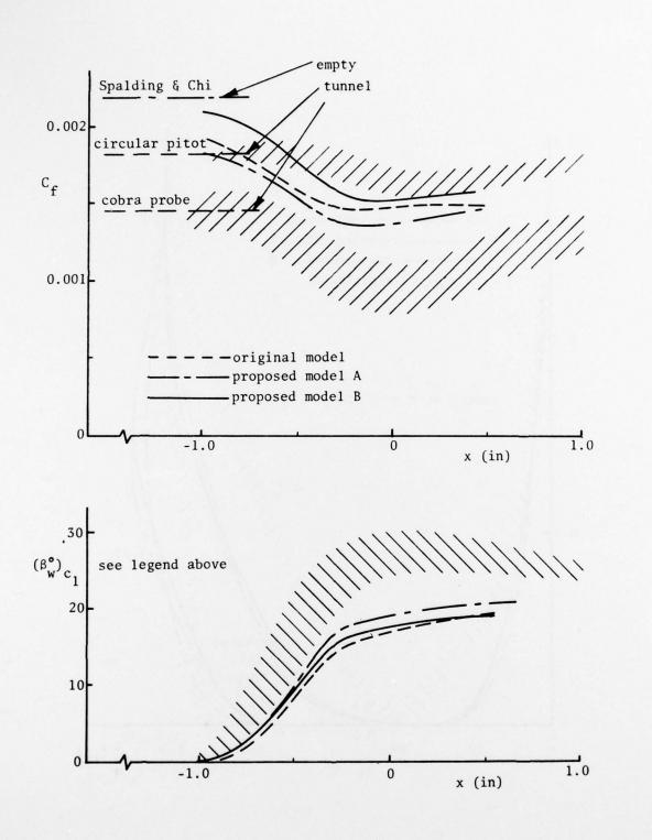
COMPARISON WITH THE DATA OF PEAKE (WALL SHEAR STRESS)
