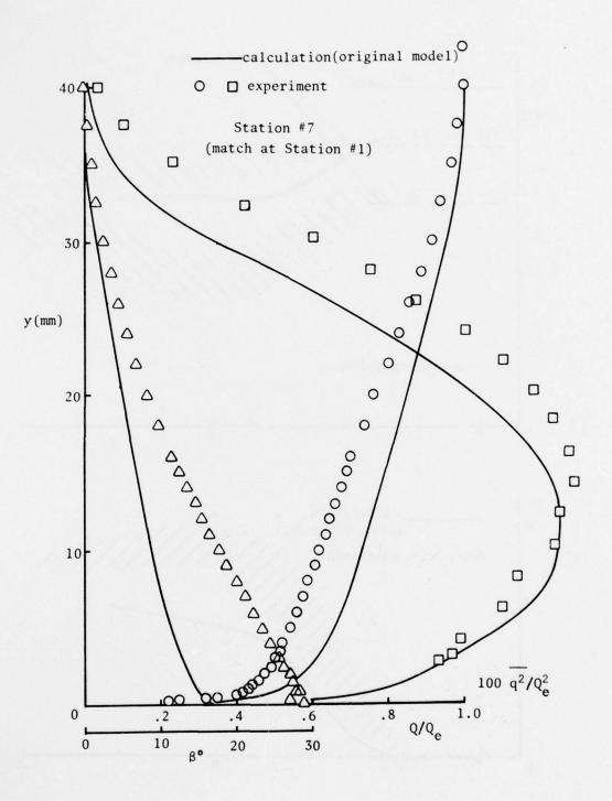
COMPARISON WITH THE DATA OF VAN DEN BERG AND ELSENAAR (VELOCITY AND  $\overline{q^2}$  PROFILES AT STATION #7)
