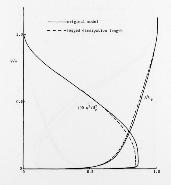
EFFECT OF REPRESENTING THE FINITE RESPONSE TIME OF THE DISSIPATION LENGTH
