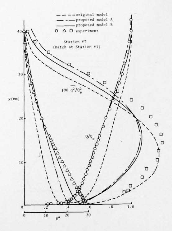
COMPARISON WITH THE DATA OF VAN DEN BERG AND ELSENAAR (VELOCITY AND  $\overline{q^2}$  PROFILES AT STATION #7)
