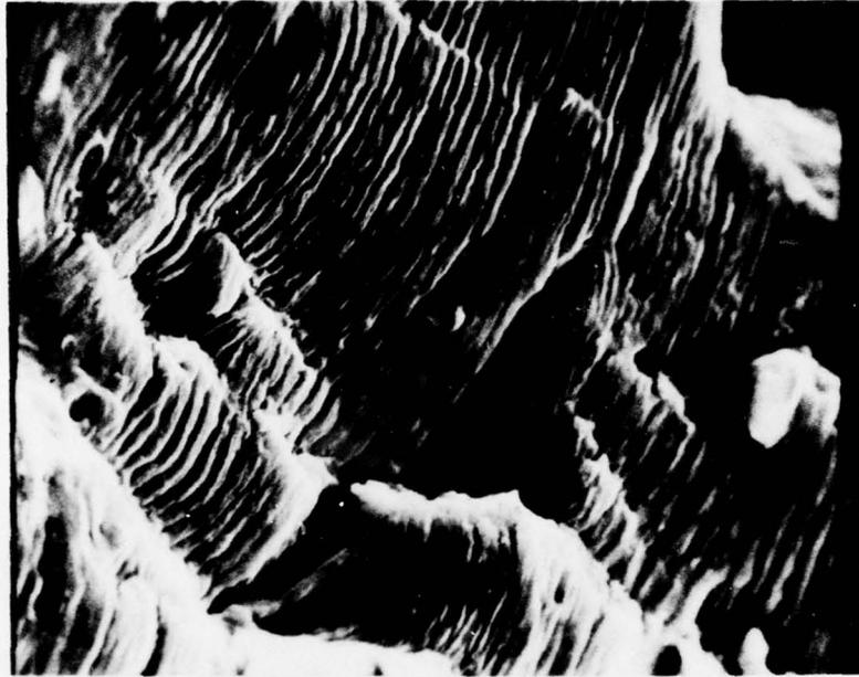
Figure 44. Fatigue striae in 5083 aluminum, 1000X.
