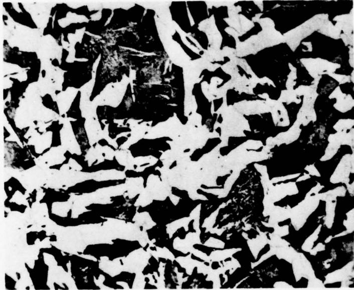
**Figure 5.** Microstructure of ASTM A-516 steel, 320X.
