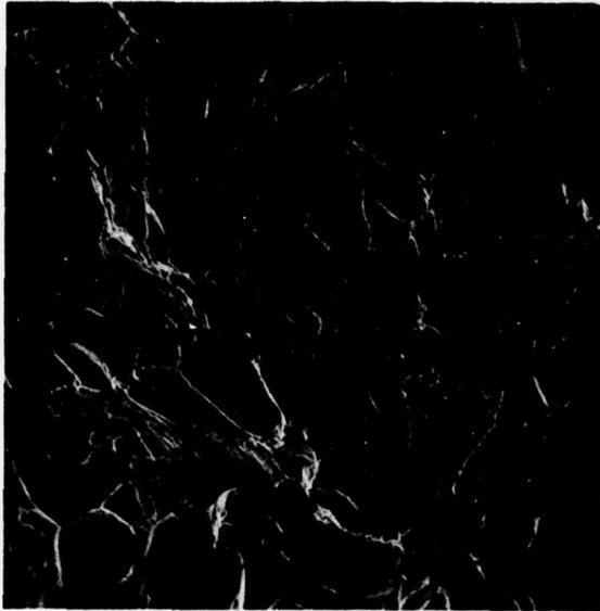
Figure 3. Typical cleavage facets, 400X.
