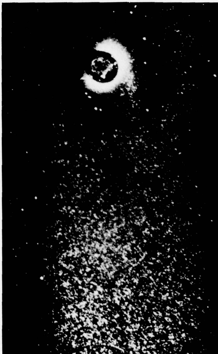
Figure 5. Small damage sites generally appear to have some form of contaminant particle fused into the surface. The small particles around the damage site are the result of partial evaporation of the contaminant particle and the glass. (50 \mu\text{m} diameter spot)
