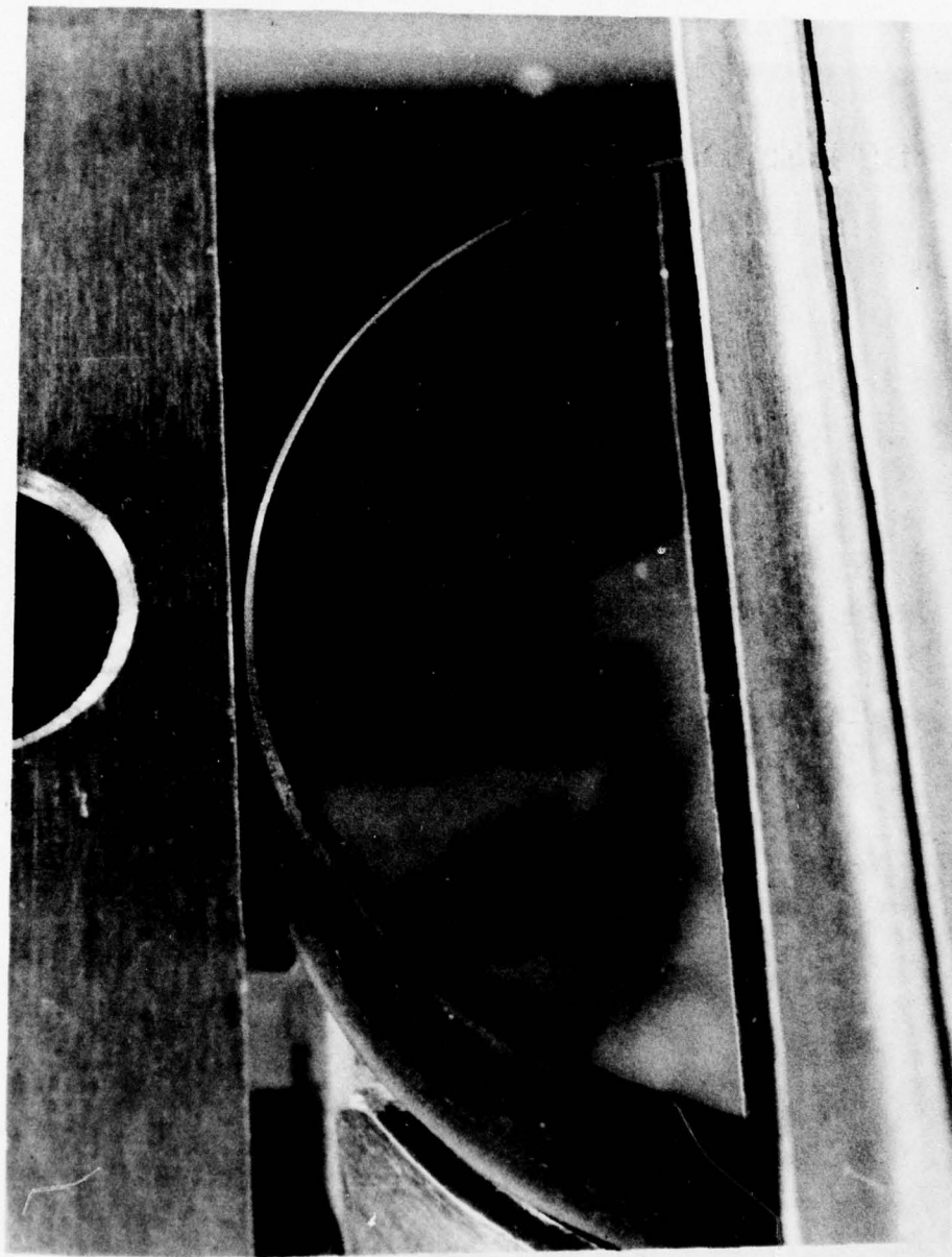
Figure 5. Site 5Cl (coating No. 5 on Cer-Vit with 1 cm diameter spot). (a) and (b), during and after a 54 \text{ J/cm}^2 exposure. (c), during 100 \text{ J/cm}^2 . (d) and (e), after 100 \text{ J/cm}^2 .
