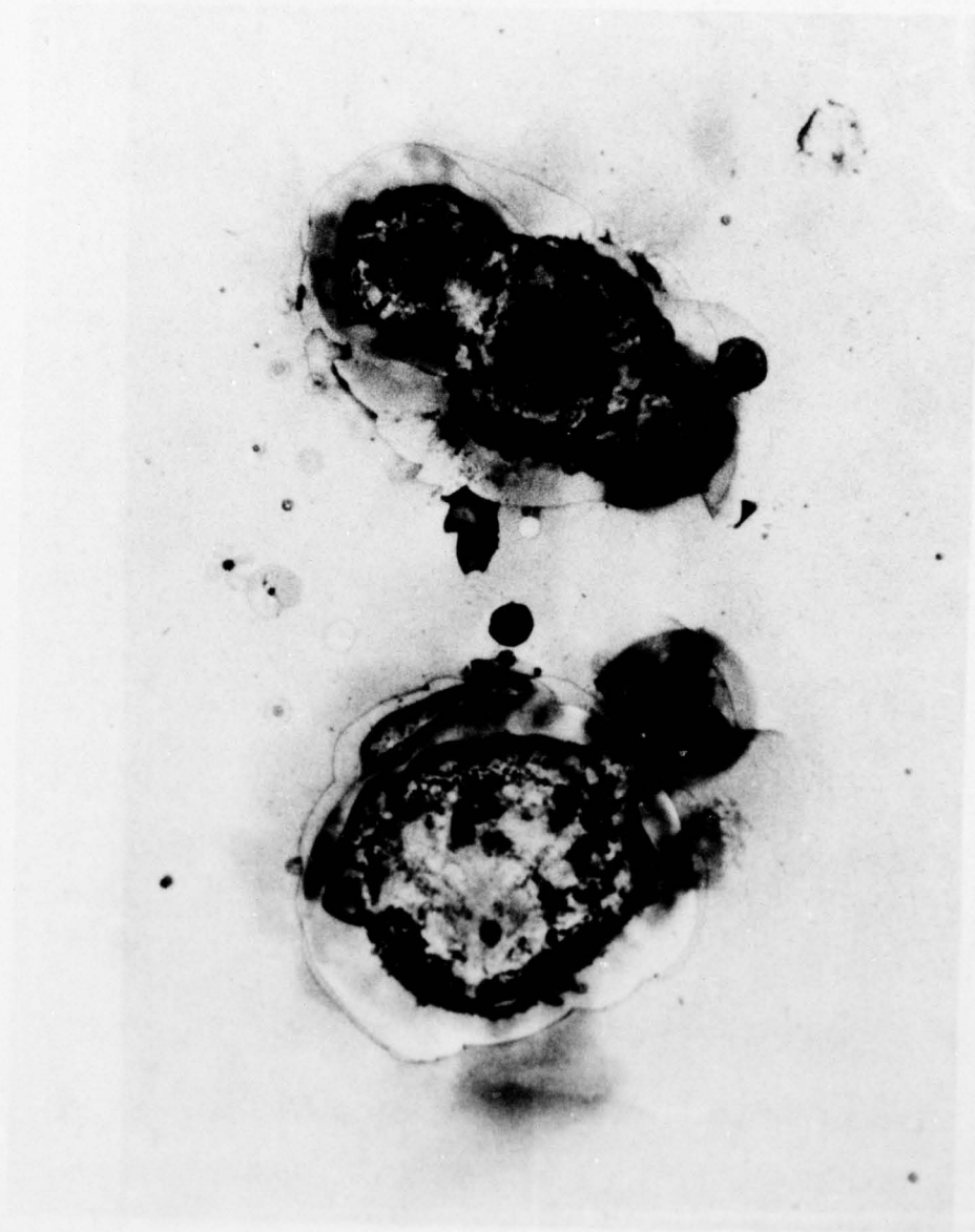
Figure 9. Brightfield (a) and Nomarski (b) views of Site 5Cs showing damage from an 84 \text{ J/cm}^2 pulse on a 0.1 \text{ cm} diameter area. The width of this micrograph is 0.1 \text{ cm} .
