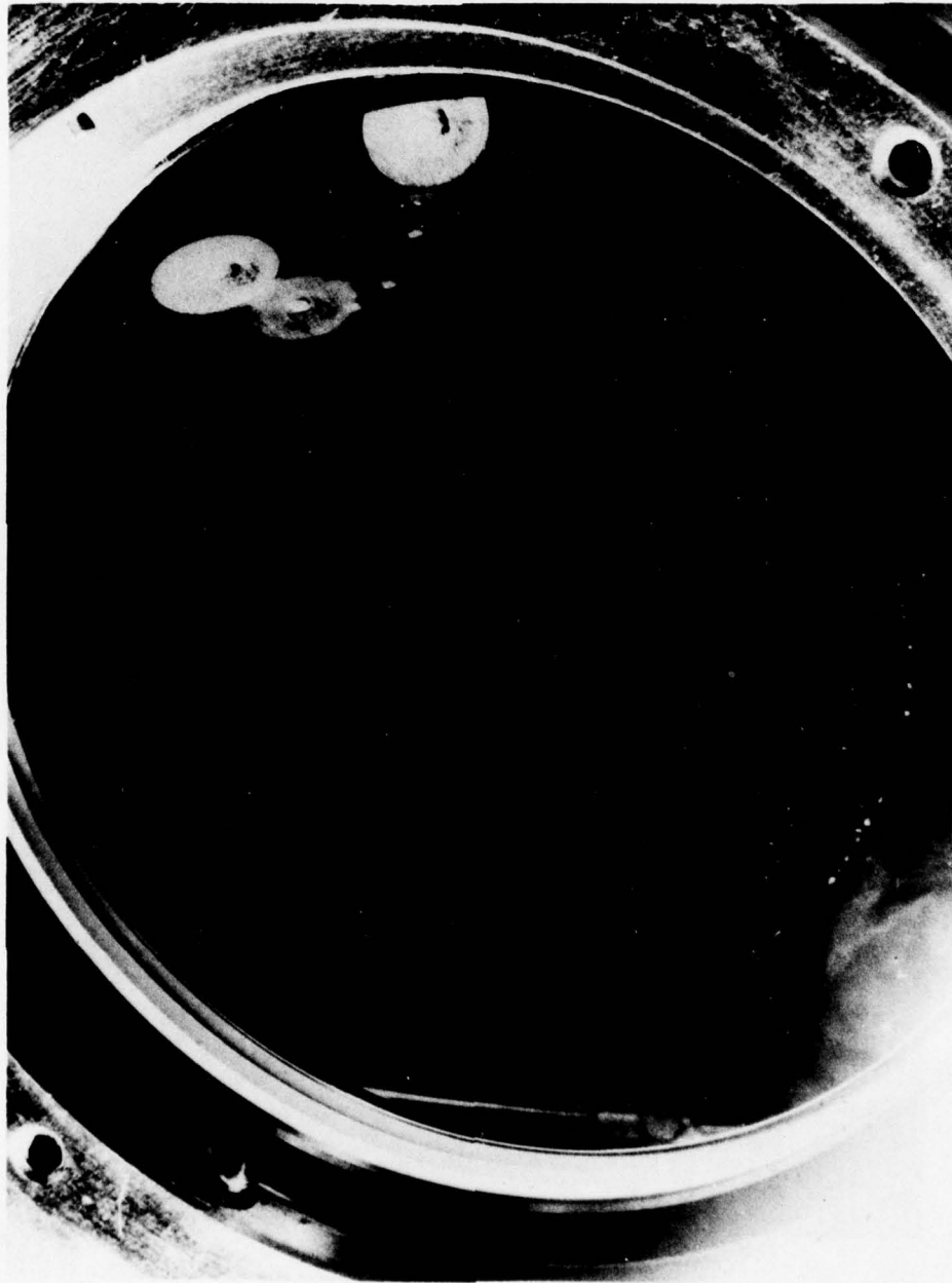
Figure 10. Antireflection coated spatial filter lens. The circular pattern of the damage follows the intensity modulations on the beam.
