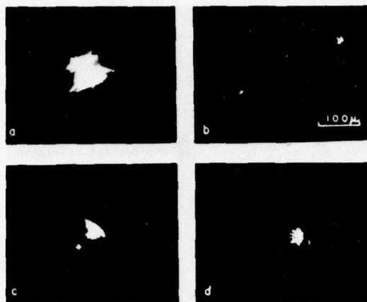
Figure 11. Light scattering observed by means of an ultramicroscope. Large clusters in (a) KBr, (b) NaCl, (c) KBr, and (d) NaCl. All crystals doped with metaborate ion. (ref. 6).
