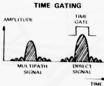
Time gating ensures that the correct signal is tracked, not the reflected one.
