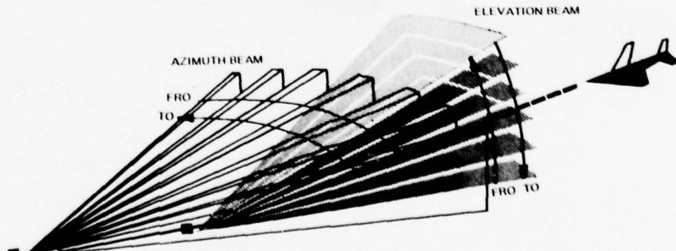
**TRSB USES A TIME-SEQUENCED SIGNAL FORMAT FOR ANGLE AND DATA FUNCTIONS.** Angle and data functions (that is, approach azimuth, elevation, flare, missed-approach guidance, and auxiliary data) are sequentially transmitted by the ground station on the same channel. Primary operation is C-band, with 300 KHz spacing between channels. However the format is compatible with Ku-Band requirements. (Note: DME is an independent function on a separate frequency and is not a part of this format.)
