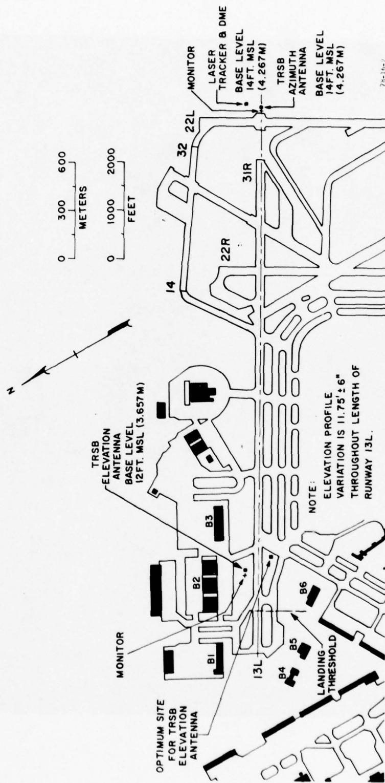
FIGURE 2. TRSB AND PRECISION LASER TRACKER SITING AT JFK RUNWAY 13L
