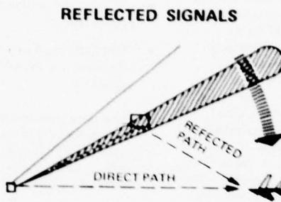
**OUT-OF-BEAM MULTIPATH.** If the angle and therefore the time between the reflected and direct beam are relatively large, the aircraft receiver is subjected to out-of-beam multipath. In this case, the TRSB processor automatically rejects the reflected signal by placing a time gate, as illustrated below, around the desired guidance signal. This ensures that the correct signal is tracked even if the multipath signal amplitude momentarily exceeds that of the desired signal.
