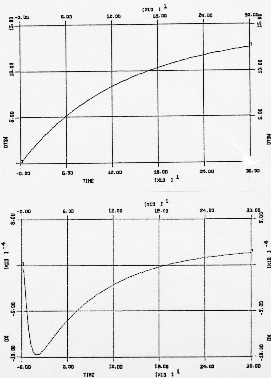
Figure 13 - SUPERHEATER WALL TEMPERATURE ( $\Delta T_{SW}$ ) VS TIME
