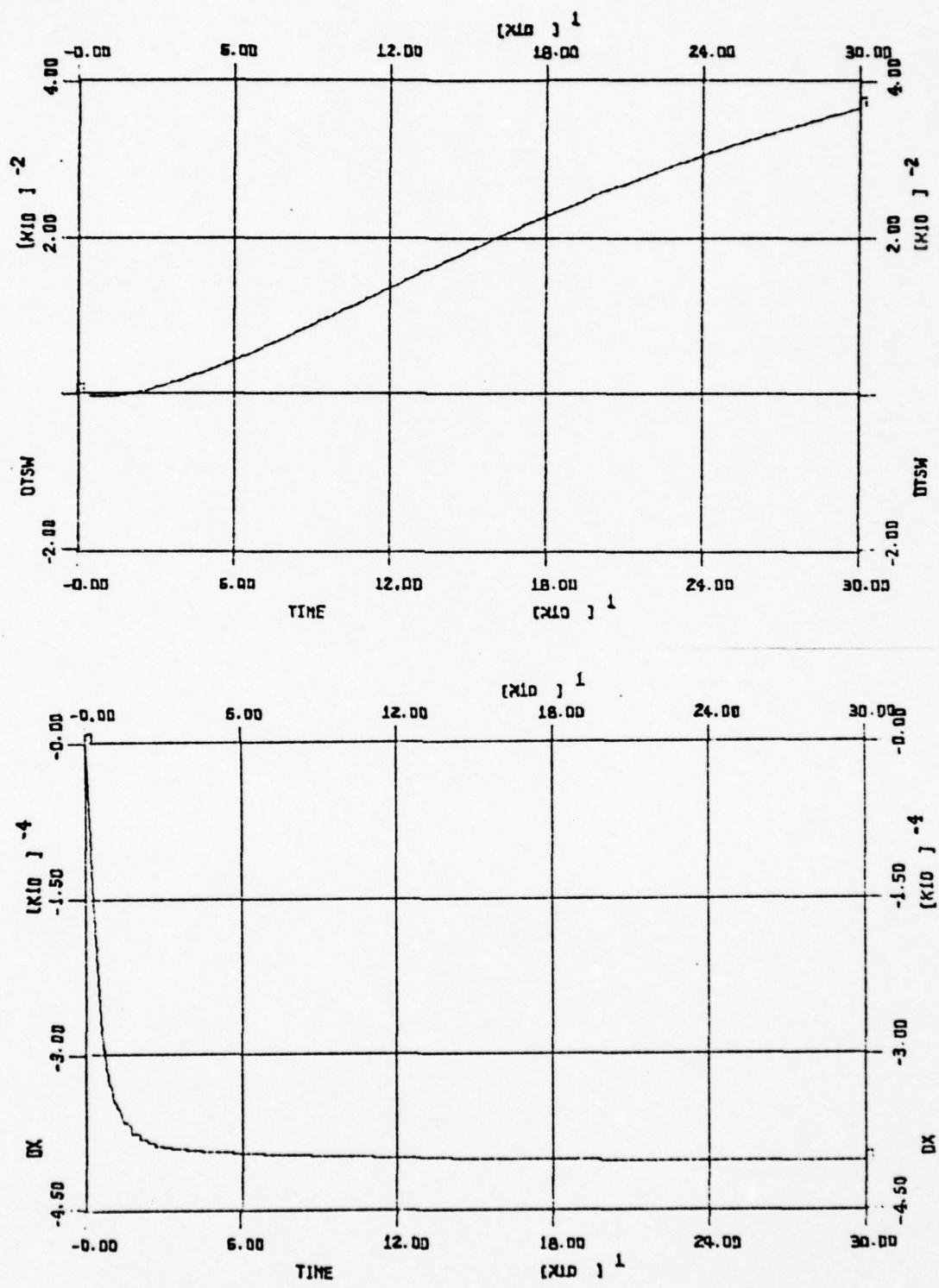
Figure 20 - SUPERHEATER WALL TEMPERATURE ( $\Delta T_{SW}$ ) VS TIME
