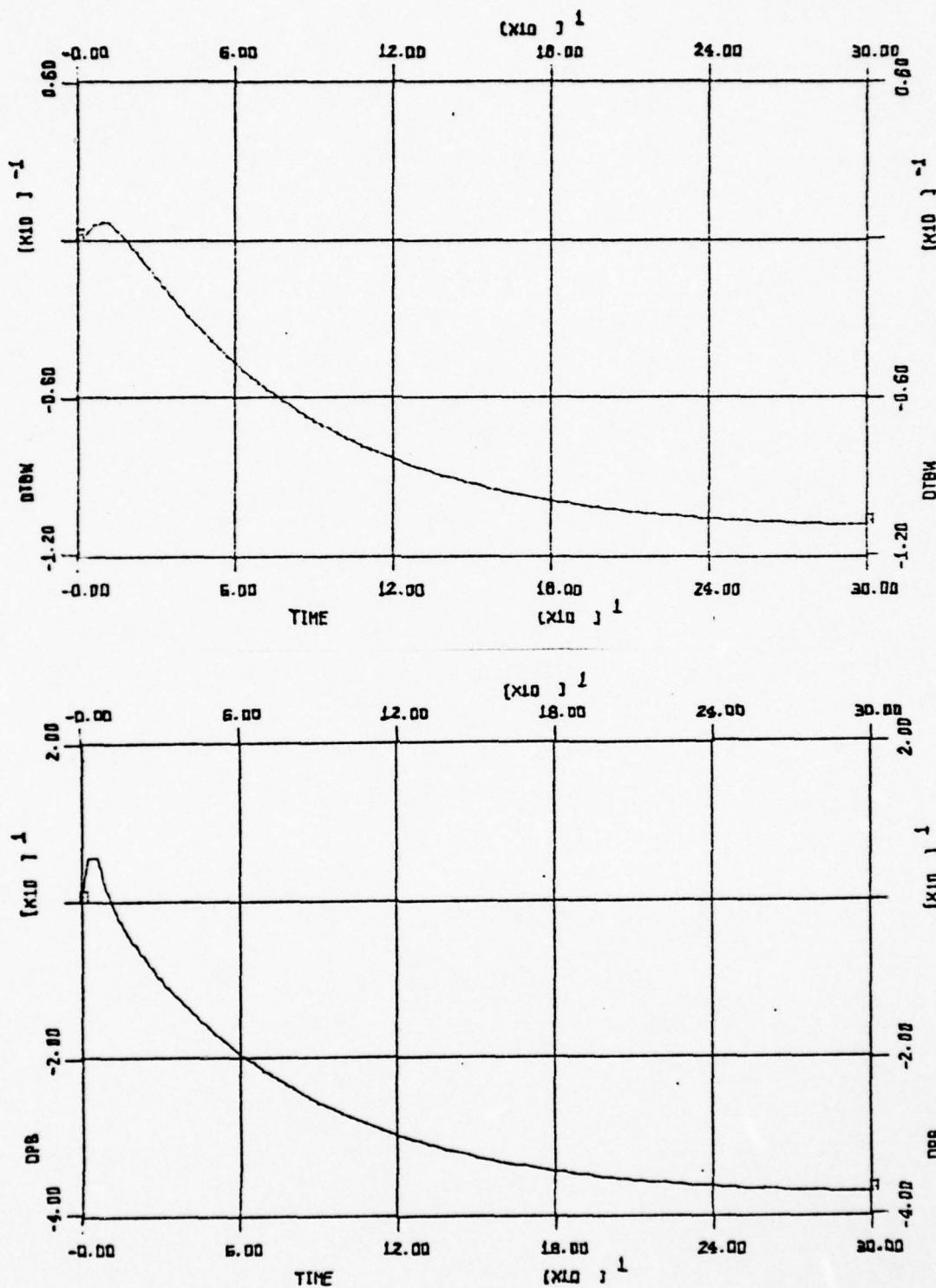
Figure 22 - RISER TUBE WALL TEMPERATURE ( $\Delta T_{BW}$ ) VS TIME
