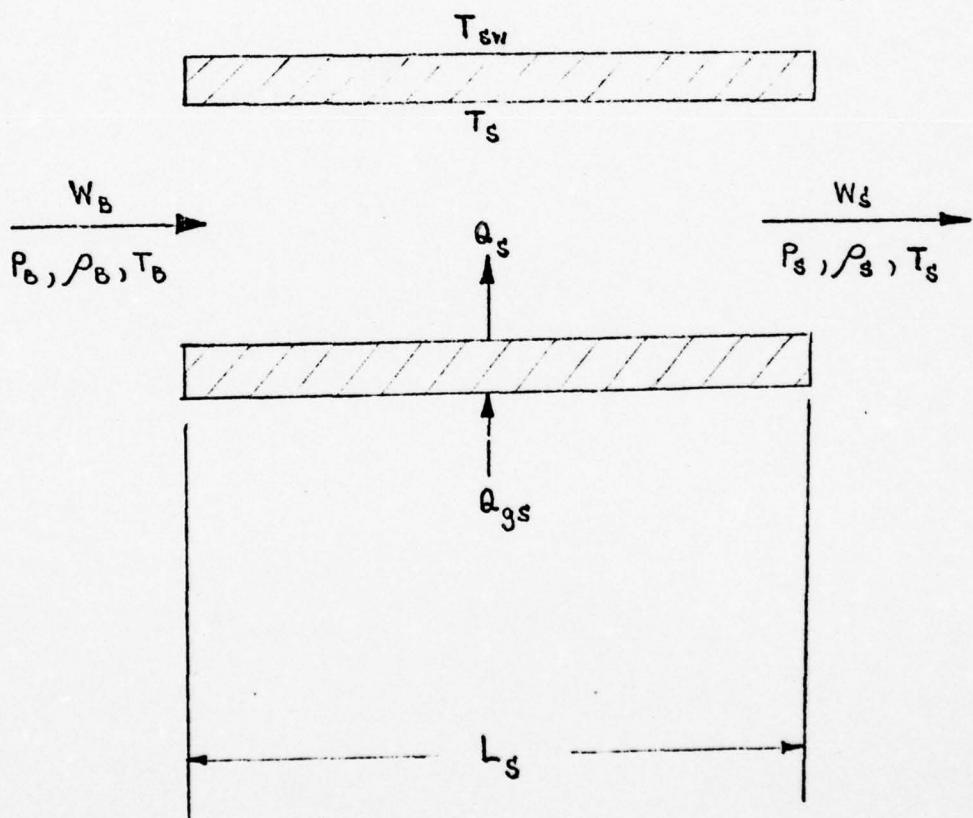
Figure 2 - SCHEMATIC DIAGRAM OF SUPERHEATER
