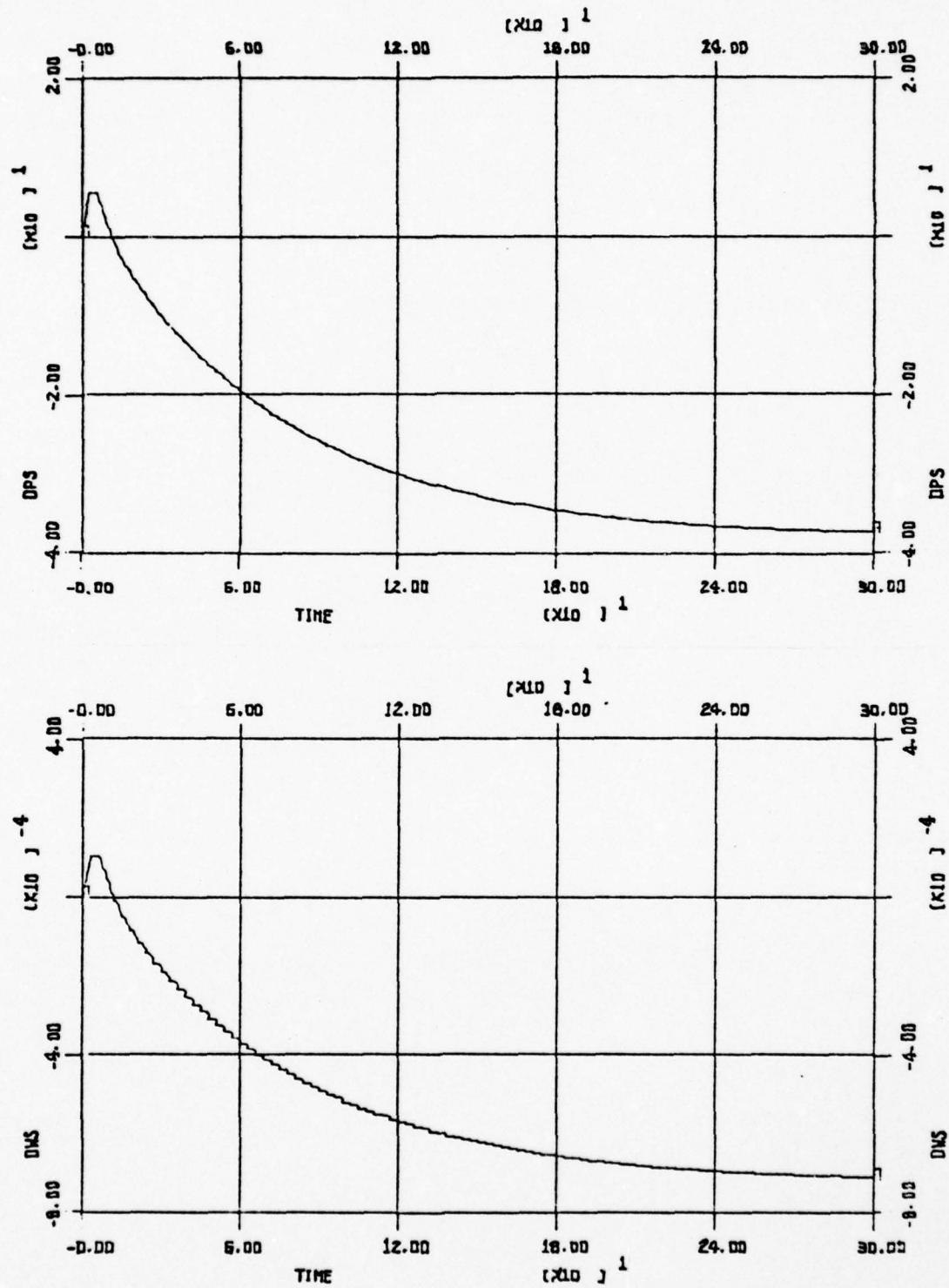
Figure 24 - SUPERHEATER OUTLET PRESSURE ( $\Delta P_s$ ) VS TIME
