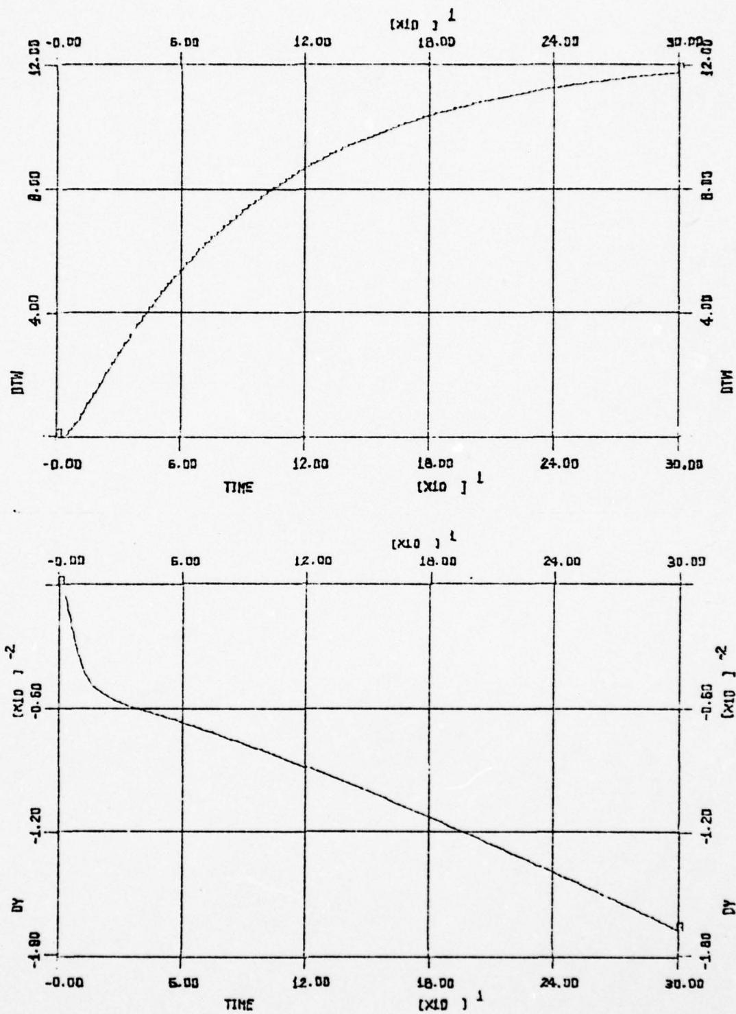
Figure 16 - STEAM DRUM LIQUID TEMPERATURE ( $\Delta T_W$ ) VS TIME
