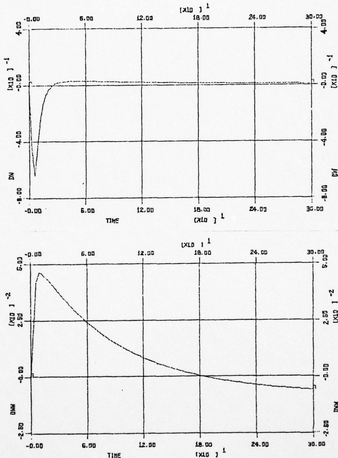
Figure 14 - RISER MIXTURE FLOW RATE ( $\Delta W$ ) VS TIME AND
