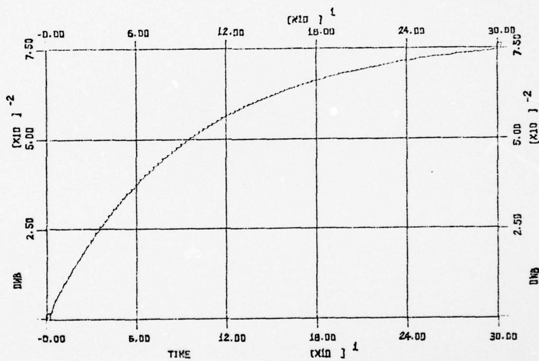
Figure 18 - STEAM MASS-FLOW RATE FROM STEAM DRUM TO SUPERHEATER ( $\Delta W_B$ ) VS TIME
