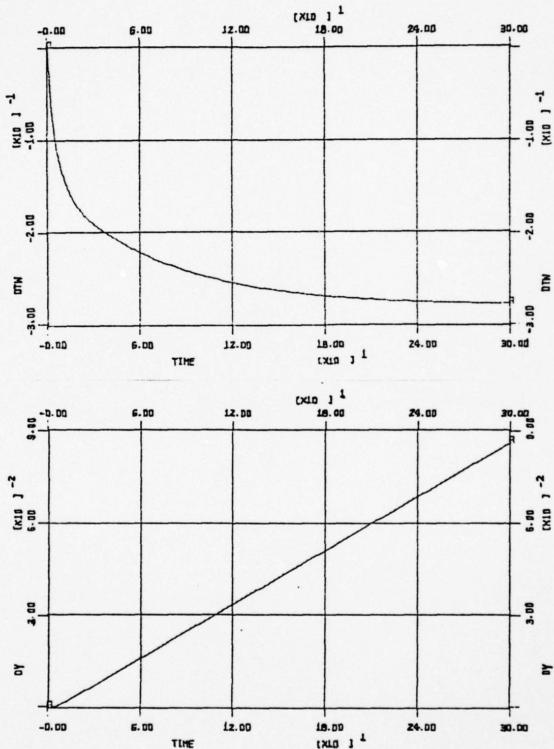
Figure 23 - STEAM DRUM LIQUID TEMPERATURE ( $\Delta T_W$ ) VS TIME
