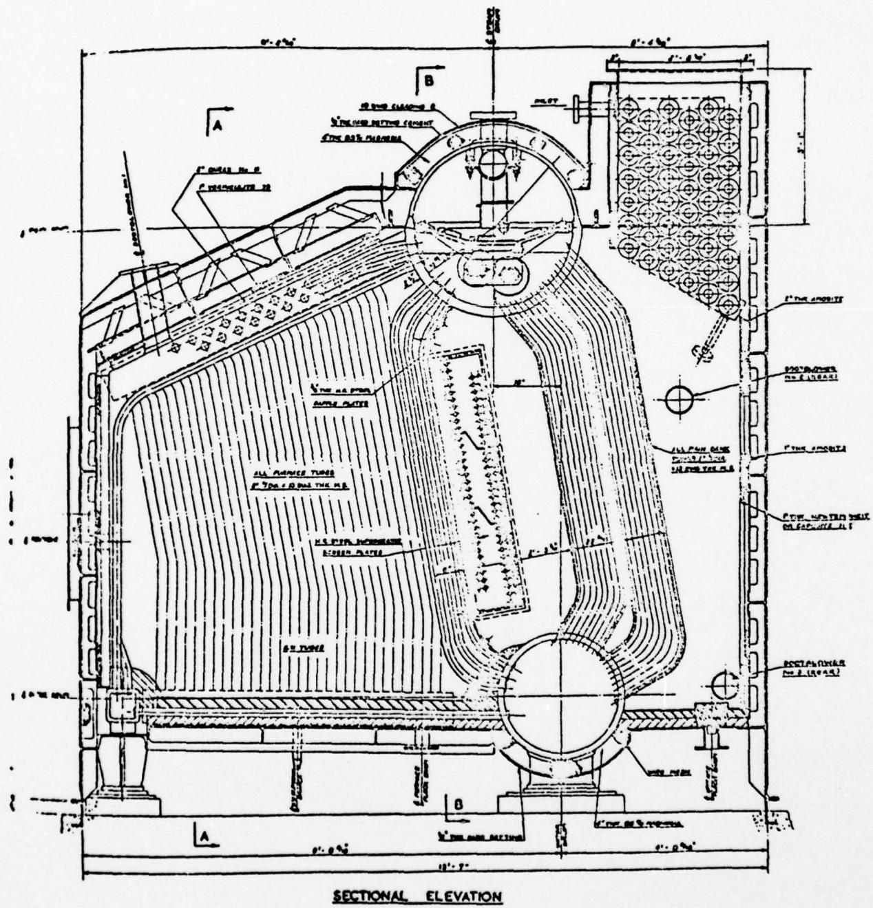
**Figure 1 - A CROSS SECTIONAL ARRANGEMENT OF THE FOSTER WHEELER D-TYPE MARINE BOILER**
