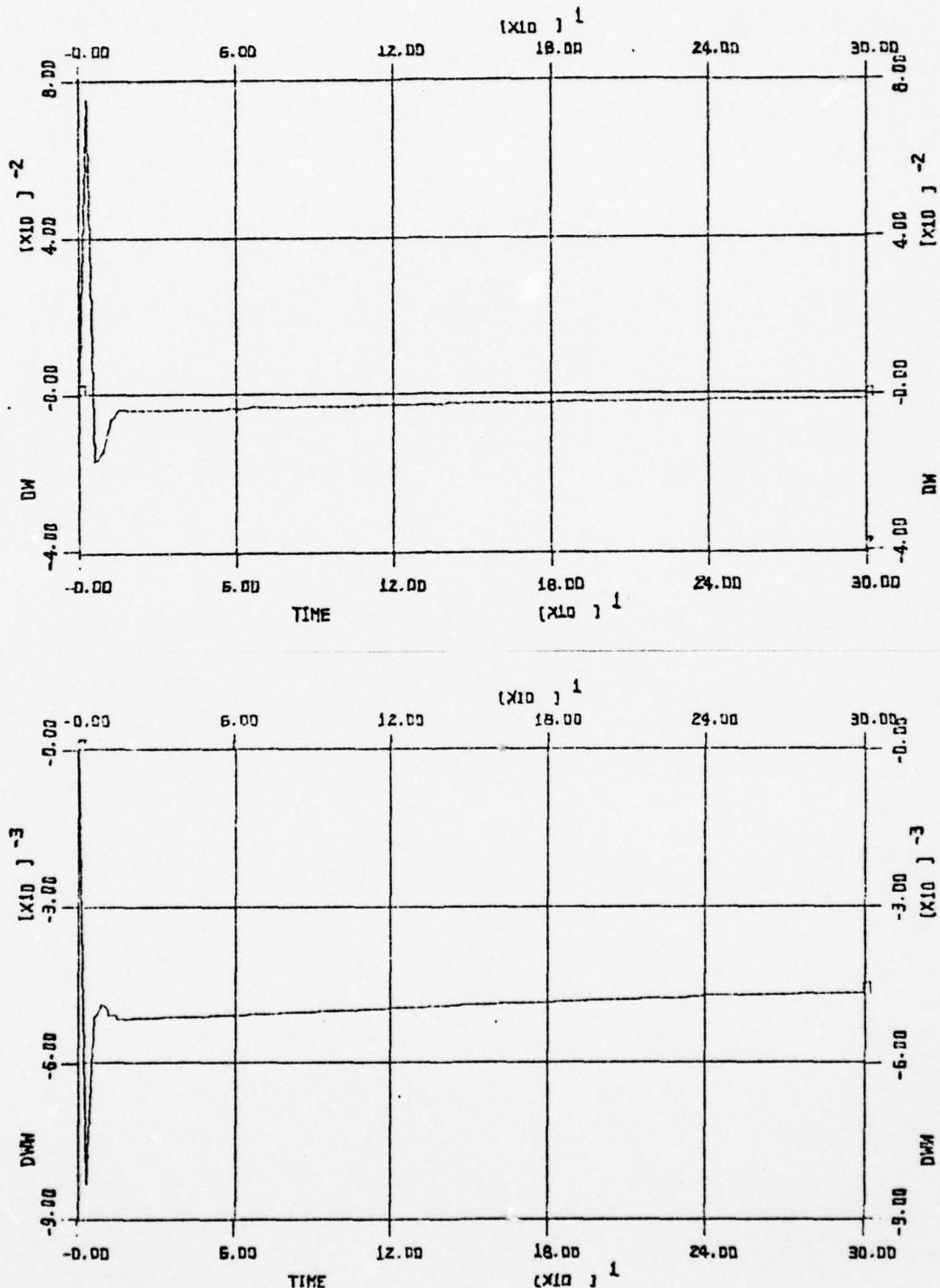
Figure 7 - RISER MIXTURE FLOW RATE ( $\Delta W$ ) VS TIME AND
