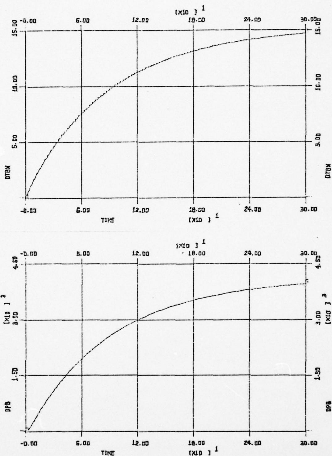
Figure 15 - RISER TUBE WALL TEMPERATURE ( $\Delta T_{BW}$ ) VS TIME
