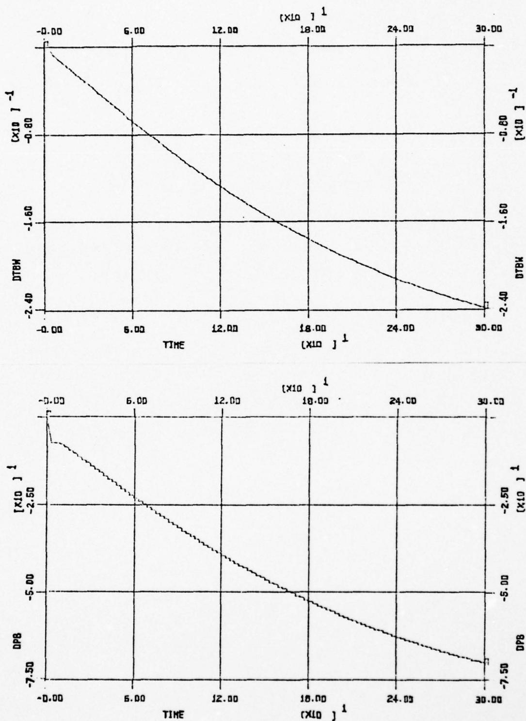
Figure 8 - RISER TUBE WALL TEMPERATURE ( $\Delta T_{SW}$ ) VS TIME AND STEAM DRUM PRESSURE ( $\Delta P_B$ ) VS TIME
