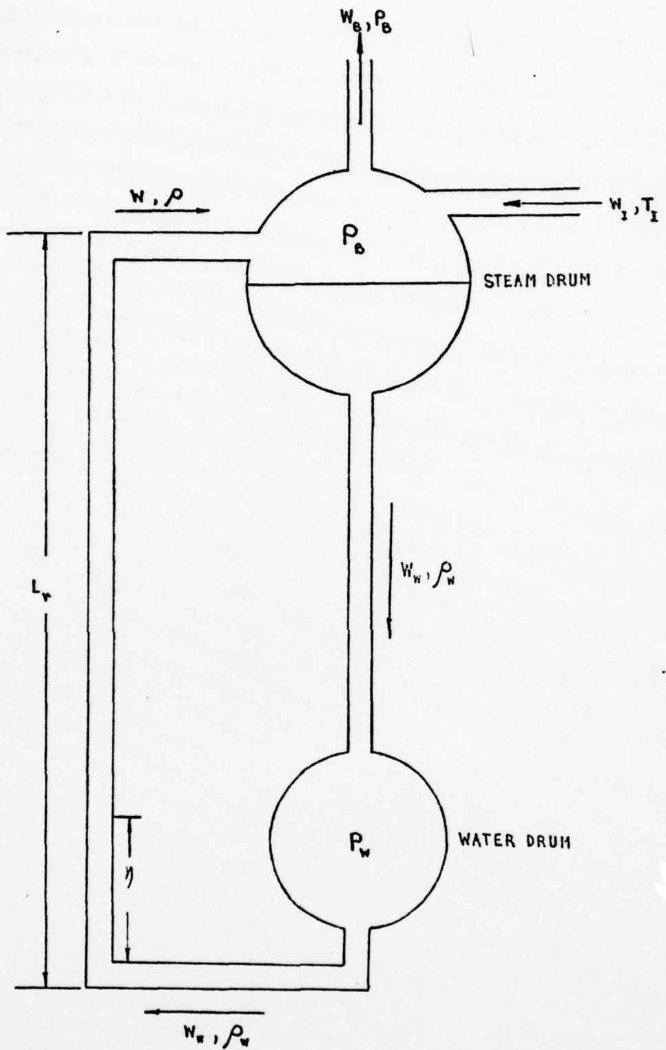
Figure 3 - SCHEMATIC DIAGRAM OF RISER-DOWNCOMER LOOP
