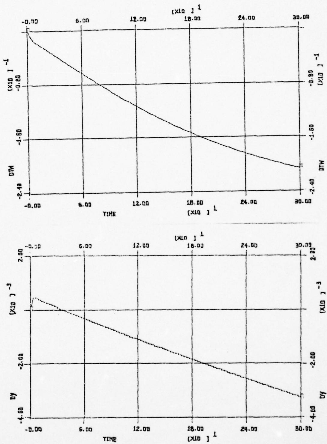
Figure 9 - STEAM DRUM LIQUID TEMPERATURE ( $\Delta T_W$ ) VS TIME
