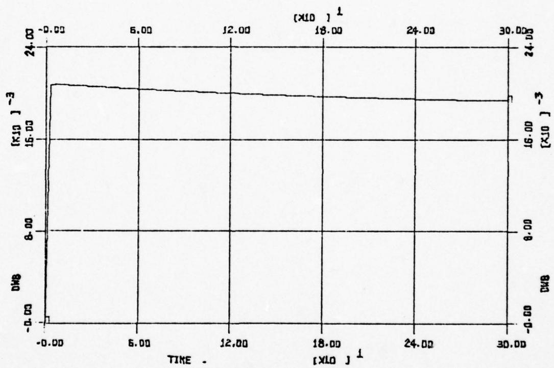
Figure 11 - STEAM MASS-FLOW RATE FROM STEAM DRUM TO SUPERHEATER ( $\Delta w_8$ ) VS TIME
