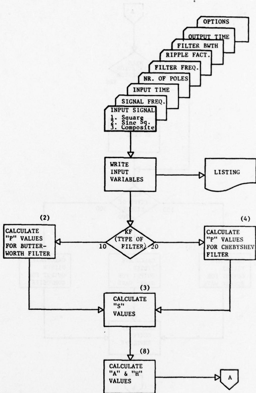
Fig. 2 Computer program functional flow diagram
