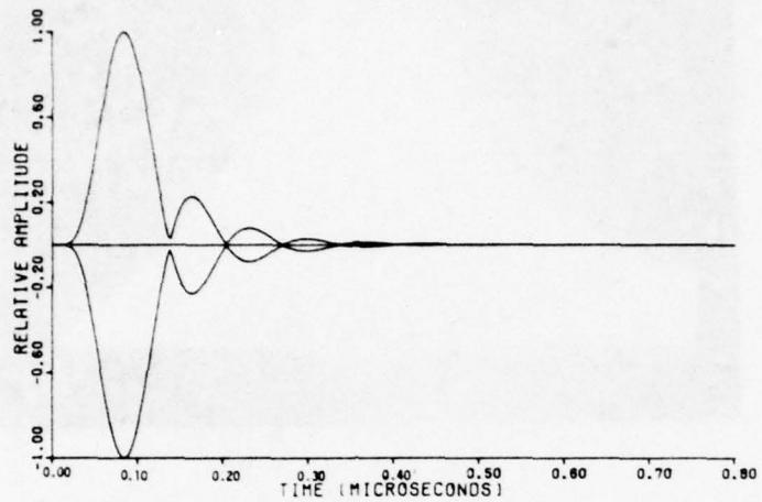
Fig. 5 Output of the 5-pole Butterworth filter with a sine squared input
