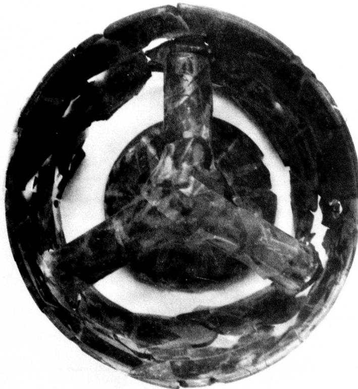
Figure 3.18 — Reconstructed Nose Cone after Failure of Rotor 1195
