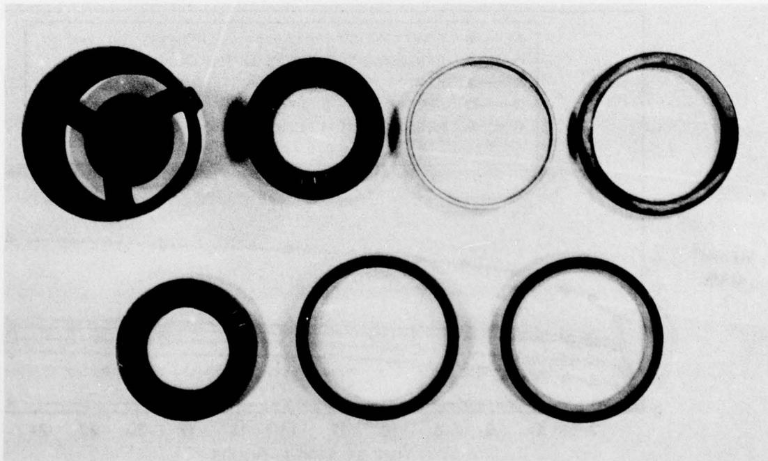
Figure 3.29 — Flowpath Components after 25 Hours at 2500°F
