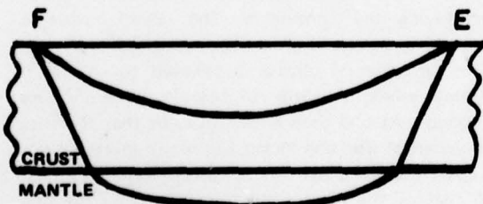
Figure 2. Direct and Refracted Rays from Focus (F) to Epicenter (E) (see text)
