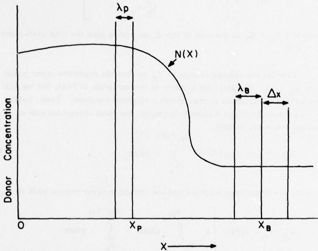
Figure 6 Schematic Diagram of Depletion Layer Positions during a Set Pulse. When the reverse bias switches from  $V_p$  to  $V_B$ , the depletion layer moves from  $x_p$  to  $x_B + \Delta x$  and then slowly settles back to the equilibrium position at  $x_B$ .
