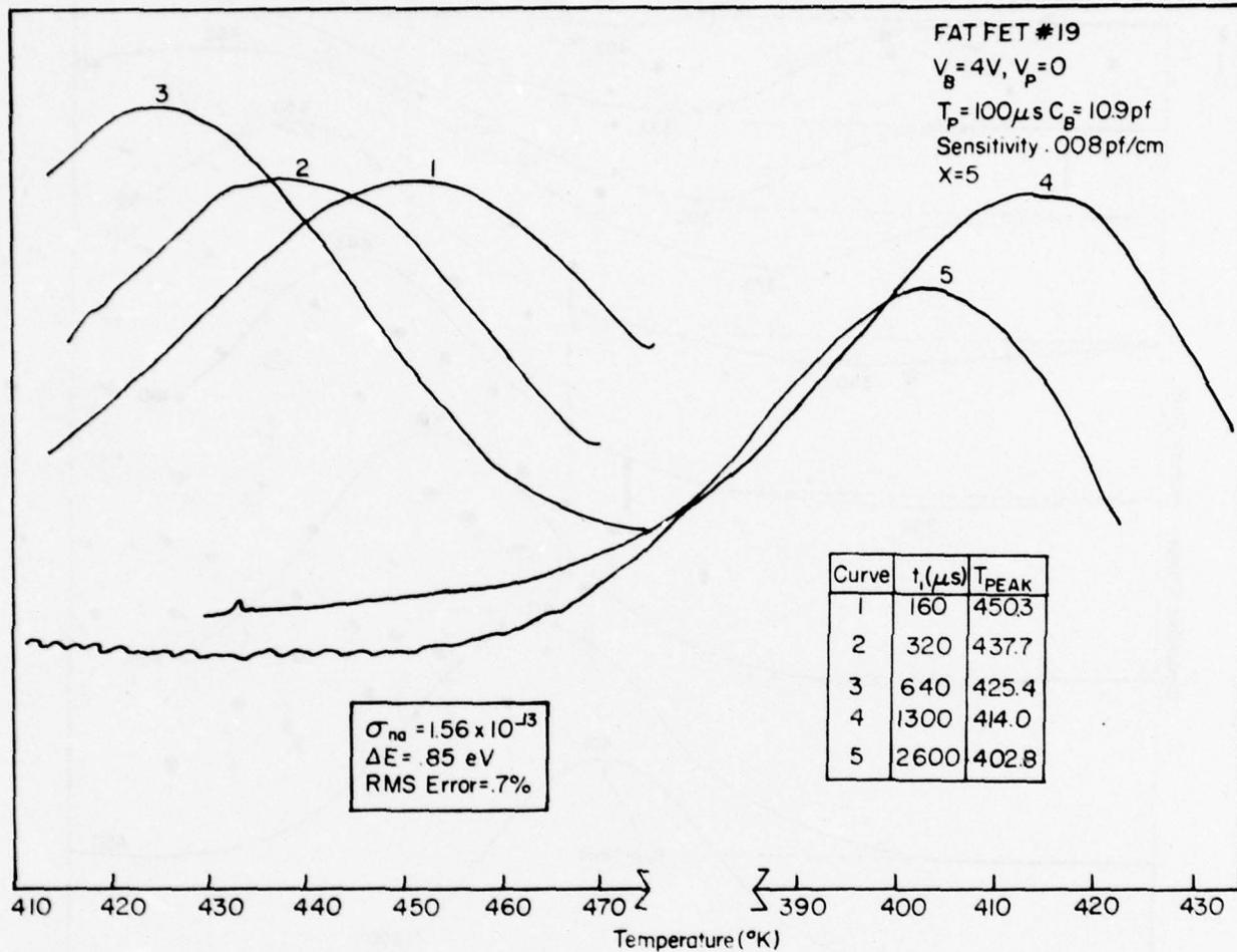
Figure 17 DLTS Curves for an Electron Bulk Trap at 0.85 eV, which has been observed by other investigators. Curves 4 and 5 are measured relative to the right-hand temperature scale which has lower temperatures than the left-hand scale which is drawn relative to curves 1-3.
