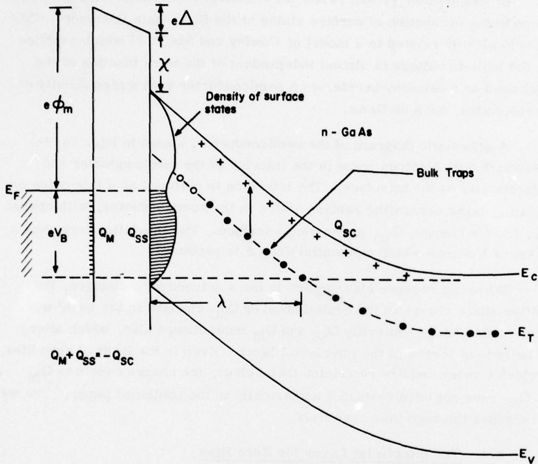
Figure 36 Schematic Diagram of Electron Trapping in the Surface States and in the bulk of the semiconductor.  $E_F$  is the Fermi level in the metal and  $V_B$  is an applied reverse bias.  $E_T$  is the bulk trap energy,  $\lambda$  is the distance to the point where the bulk trap level crosses the Fermi level,  $\chi$  is the electron affinity,  $\phi_m$  is the metal work function and  $\Delta$  is the potential drop across the interfacial layer.
