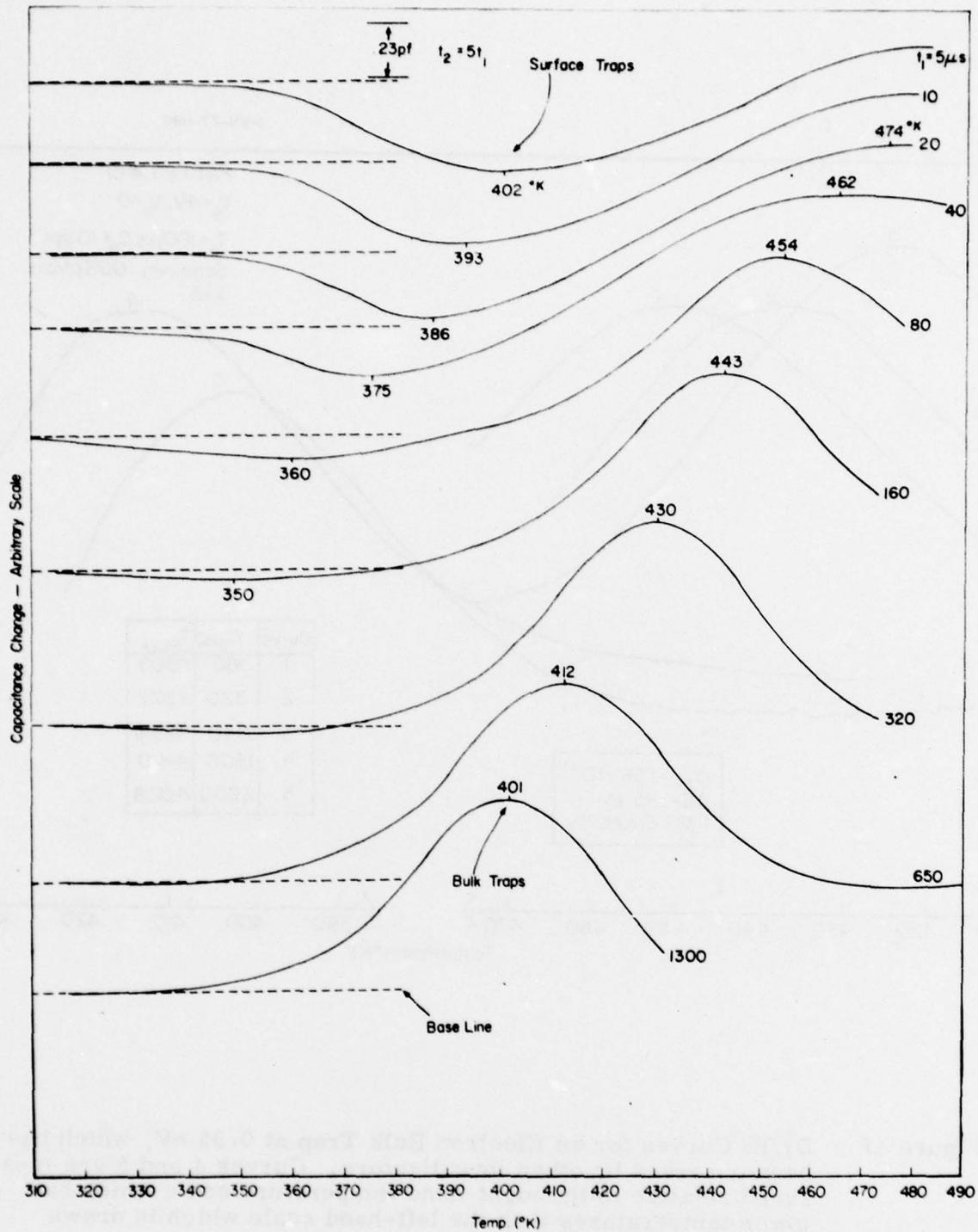
Figure 18 DLTS Curves for Values of the Boxcar Times  $t_1$  Ranging from 5 to 1300  $\mu\text{s}$ . A positive peak corresponding to the oxygen bulk trap appears at the high temperature end of curves 3-9. Negative peaks, which we associate with surface states, appear at lower temperatures and can be distinguished on the first six curves.
