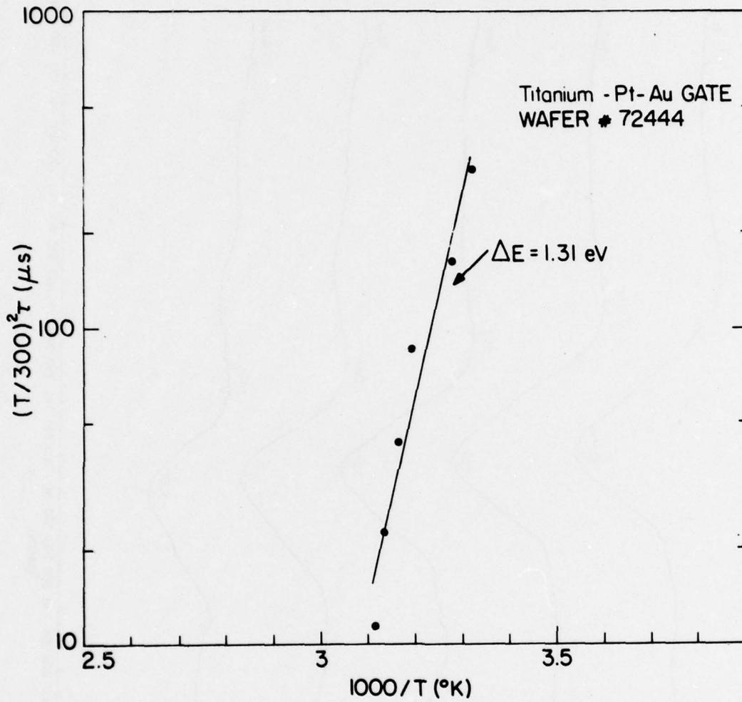
Figure 35  $(T/300)^2$  Times the Relaxation Time for a Surface Trap Under a Ti-Pt-Au gate, plotted versus  $1000/T$ . The straight line with a slope corresponding to  $E_{na} \approx 1.31 \text{ eV}$  is a least squares fit with an error of 22 percent.
