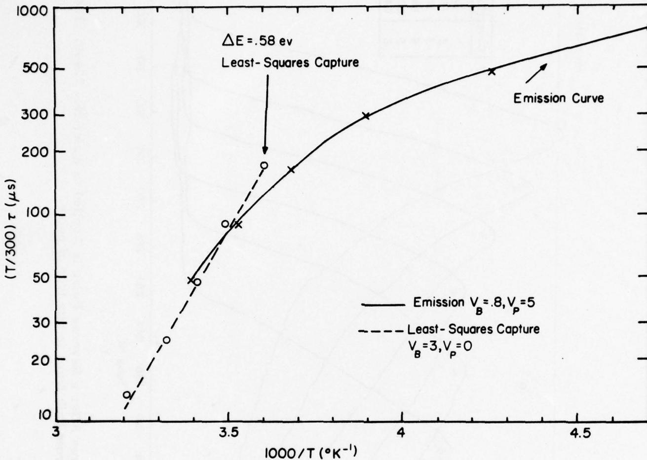
Figure 30 Relaxation Times from Set Pulses (Capture Rates) and Reverse pulses (emission rates) for the surface states detected on fat FET No. 12. The capture times fall along a straight line in the same way as for bulk traps. The emission times fall along a curve, although they could be represented fairly well by two straight lines, through the 3 high temperature and 3 low temperature points.
