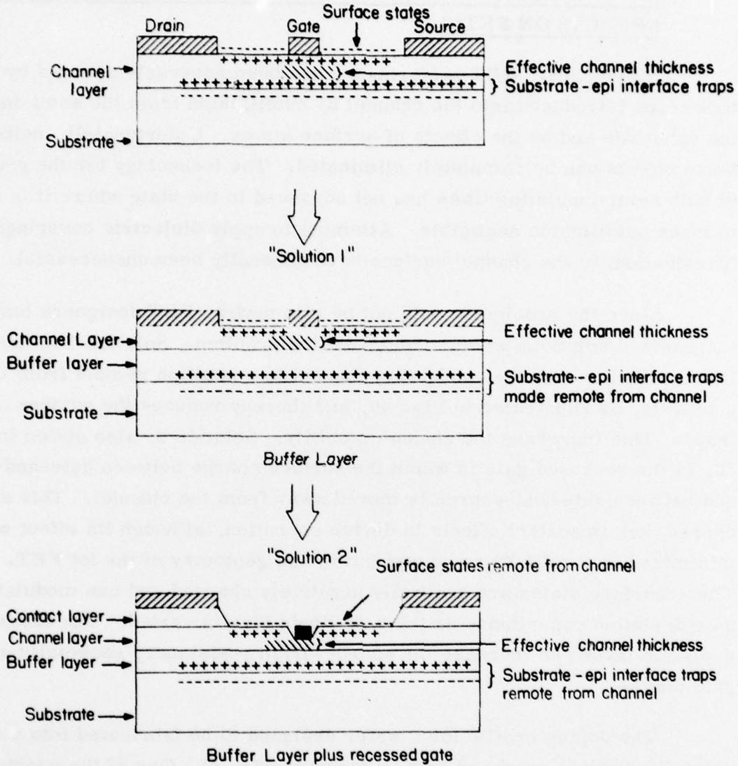
Figure 40 Chronological Sequence of Changes in Device Technology to Minimize Effects of Traps.
