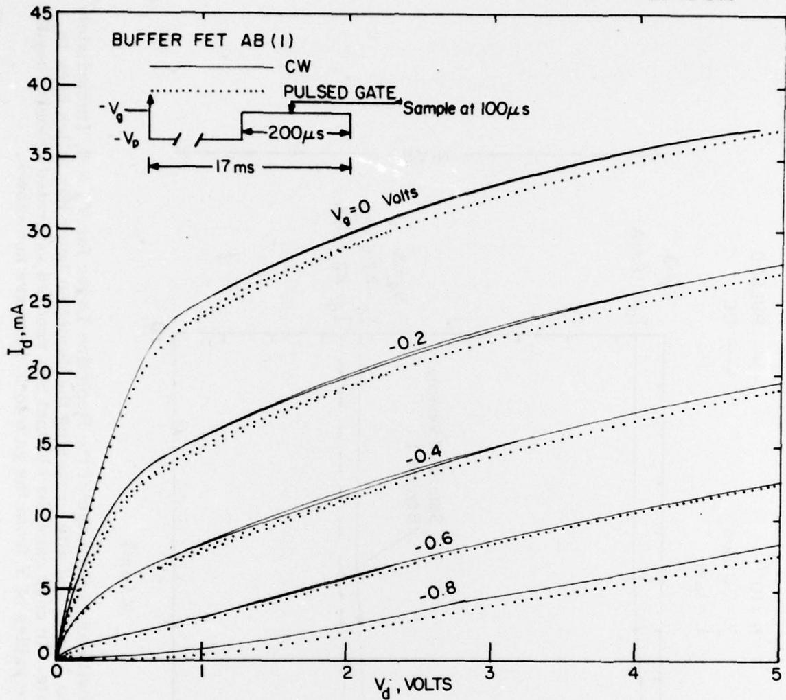
Figure 47 The DC and Pulsed Drain Characteristics of the Buffered Transistor. The gate is pulsed from pinchoff value to the indicated value. The change in the characteristics indicate the depletion layer is shrinking, as would be expected for surface states under the gate recovering from a reverse pulse.
