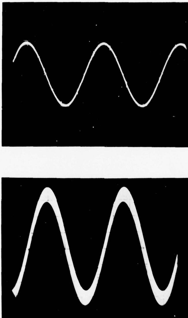
**Figure 9** Cyclical Response of Measured Capacitance due to a 100Hz rf voltage imposed on a 35 volt reverse-biased diode
