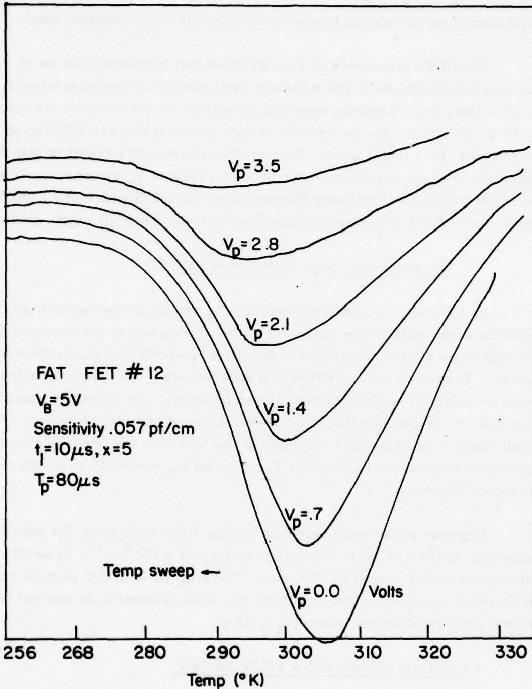
Figure 32 DLTS Signals after the Voltage is Pulsed back to Different Values of  $V_p$  with  $V_B$  fixed at 5 Volts. As the pulse-back voltage  $V_p$  approaches zero bias, more surface states are emptied as the signal amplitude increases. As  $V_p$  decreases, the maximum response occurs at higher temperatures indicating a different time constant.
