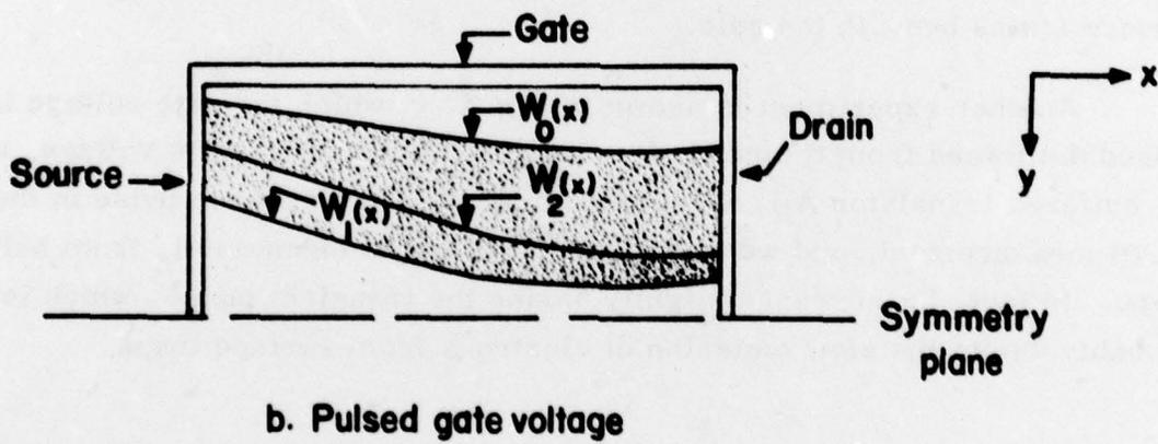
Figure 45 Schematic Diagram of a Depletion Layer in a FET During a trap setting pulse ( $W_1(x)$ ), immediately after the pulse ( $W_2(x)$ ) and after the FET has had time to reach a new steady state.
