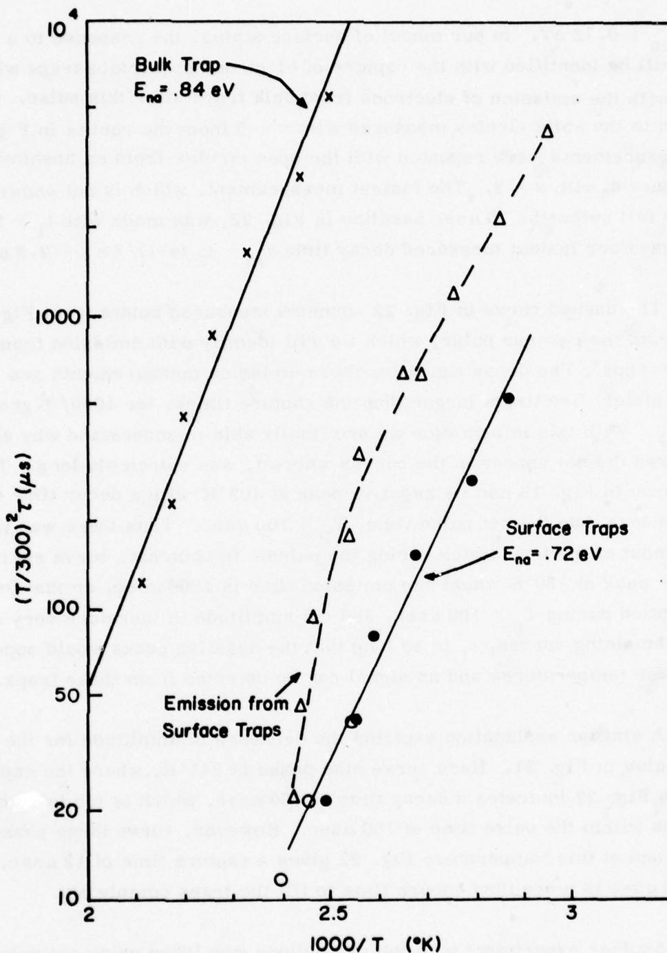
Figure 22 Plots of  $(T/300)^2 \tau$  versus  $1000/T$ . The upper straight line is a least squares fit for a bulk electron trap. The lower straight line with  $E_{na} = 0.72 \text{ eV}$  is due to capture of electrons by surface states after the set pulses in Fig. 18. The dashed curve connects points calculated from the reverse pulse data in Fig. 21 which are caused by emission from surface traps.
