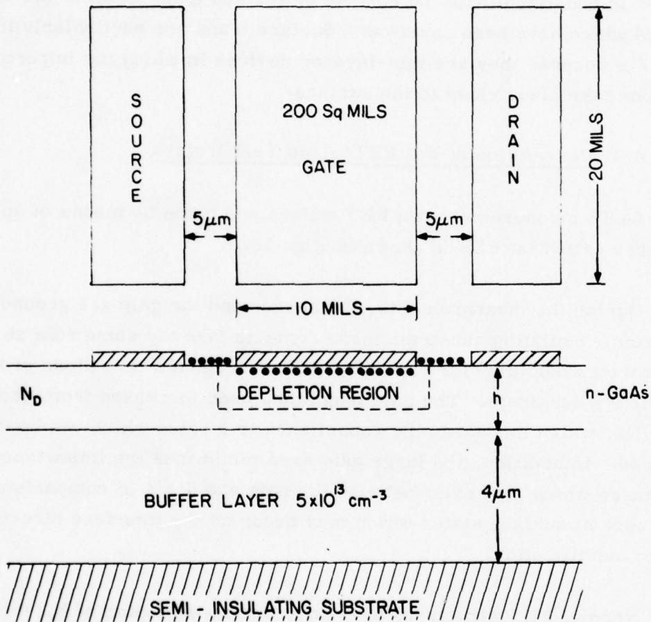
Figure 16 Structure of a Fat FET. The top view shows the dimensions of source gate and drain contacts. The side view shows a buffer layer between the semi-insulating substrate and the active layer.
