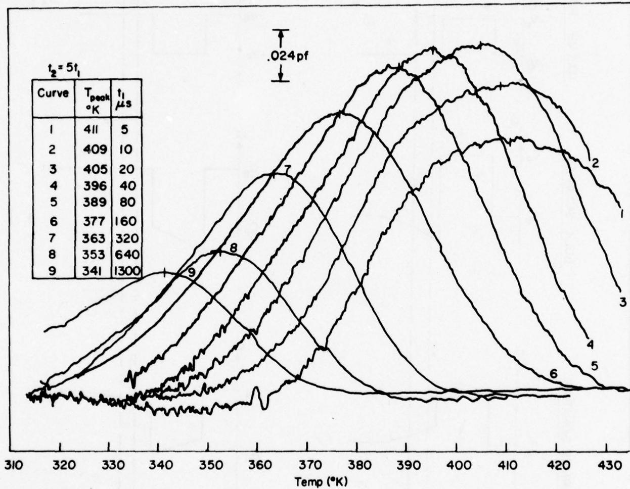
Figure 21 DLTS Curves From Surface States for a Reverse Pulse with  $V_B = 0$  and  $V_p = 20$  when the pulse length  $T_p$  is  $100 \mu s$ .
