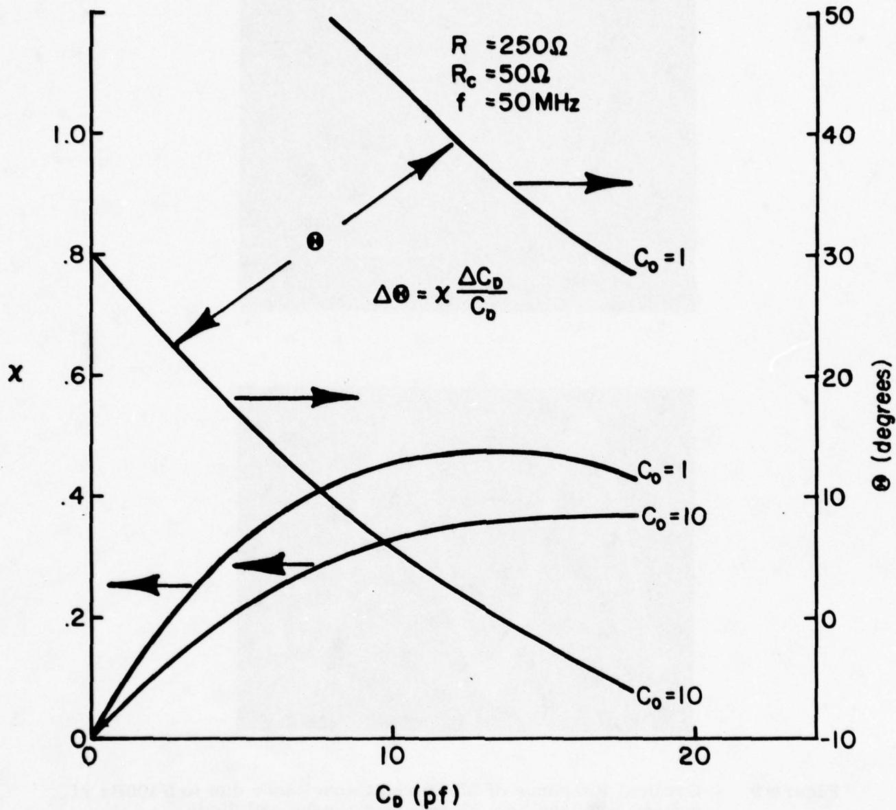
Figure 8 Plot of  $\theta$ , the Phase Change (in degrees) Induced by the Device Capacitance  $C_D$  and the differential phase change (in radians) caused by a fractional change  $\Delta C_D / C_D$  in the device capacitance.
