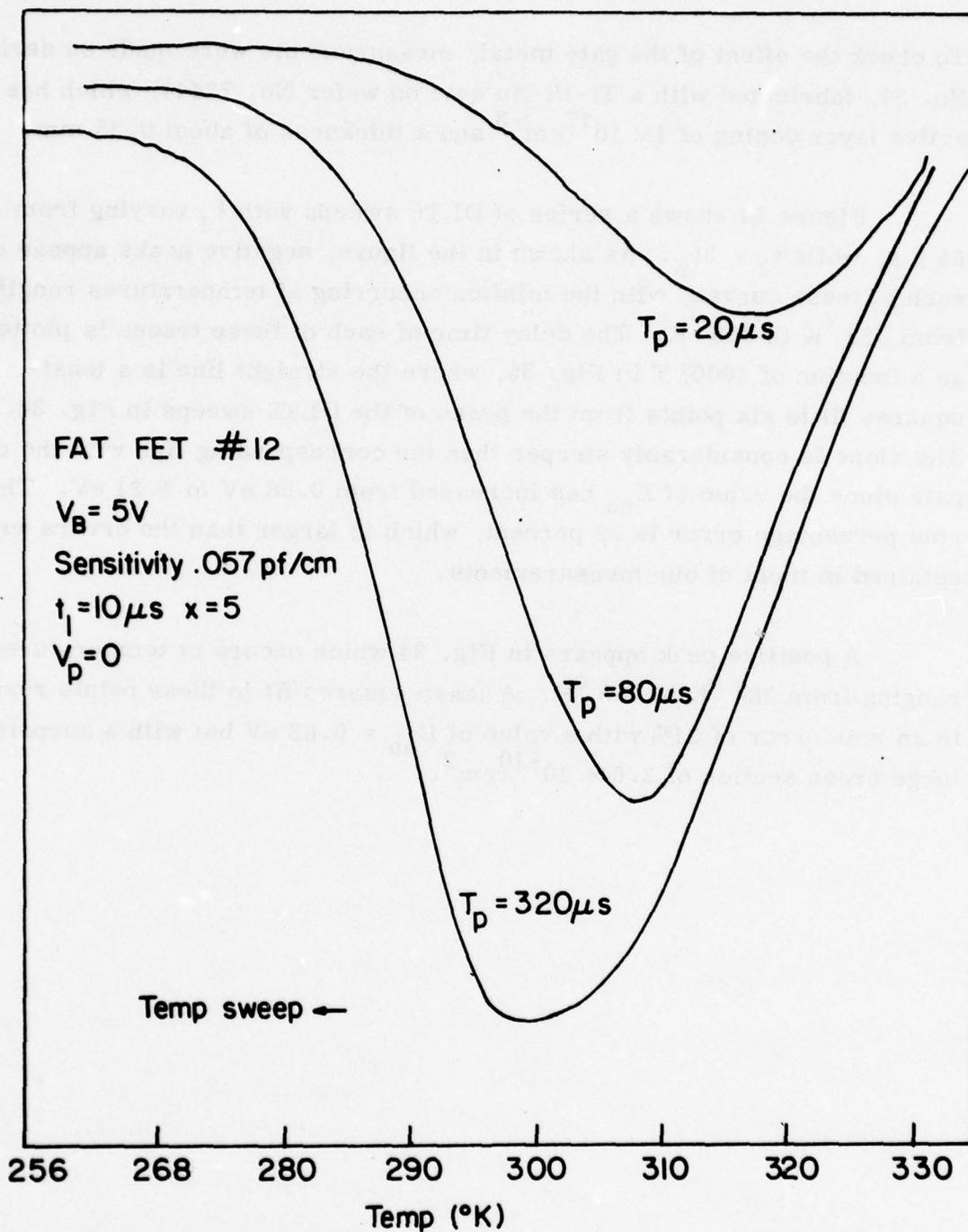
Figure 33 The Effect of increasing  $T_p$  in a Set Pulse. The surface states are slow to empty since they require about one hundred microseconds to reach full amplitude. There is a decrease in temperature of the peak response as  $T_p$  increases, suggesting that the trap states which are slowest to fill are the most rapid to empty.
