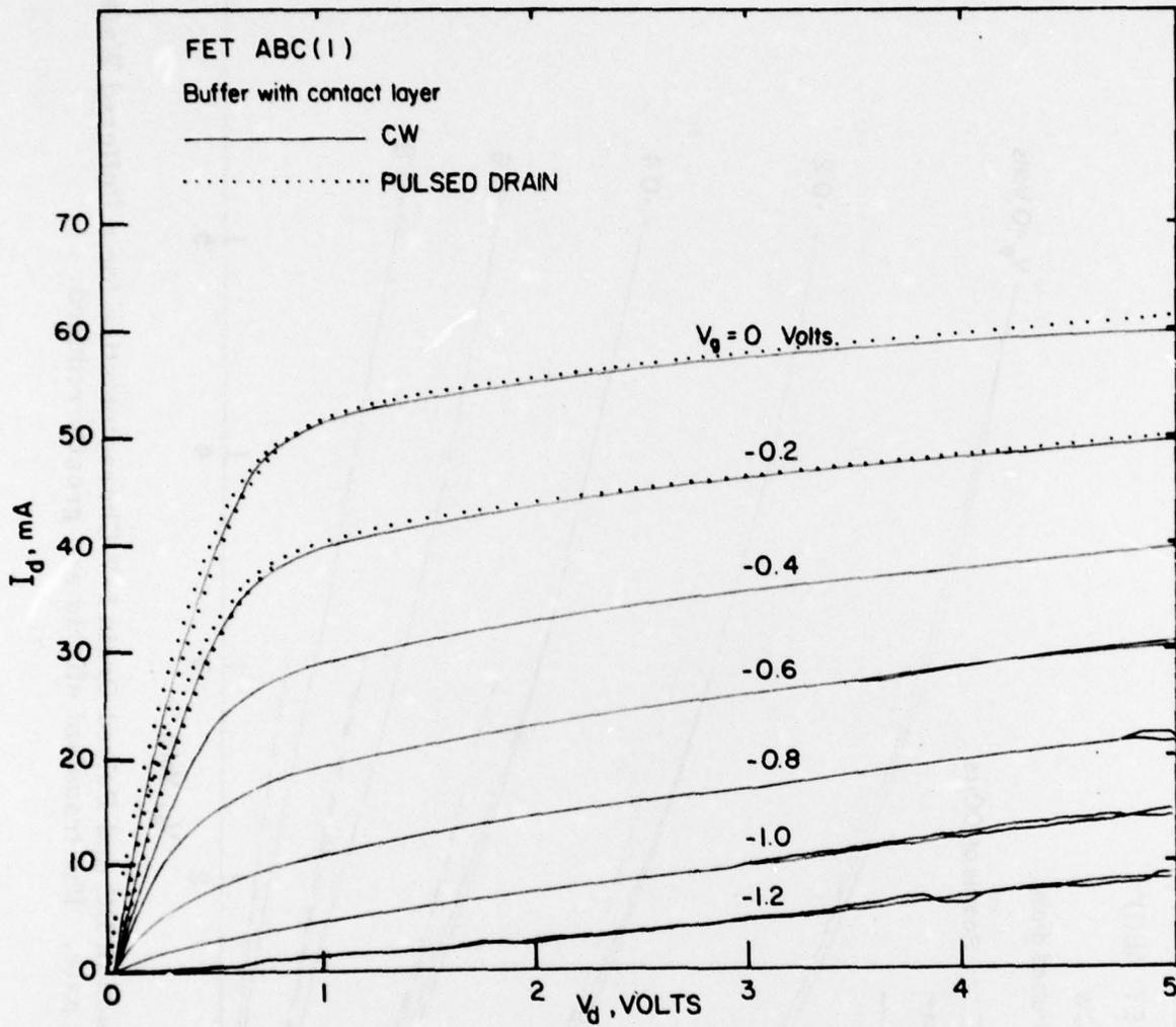
Figure 44 Comparison of DC and Pulsed Drain Characteristics for a Wafer with both Buffer and Contact Layer. The transient effects are nearly eliminated.
