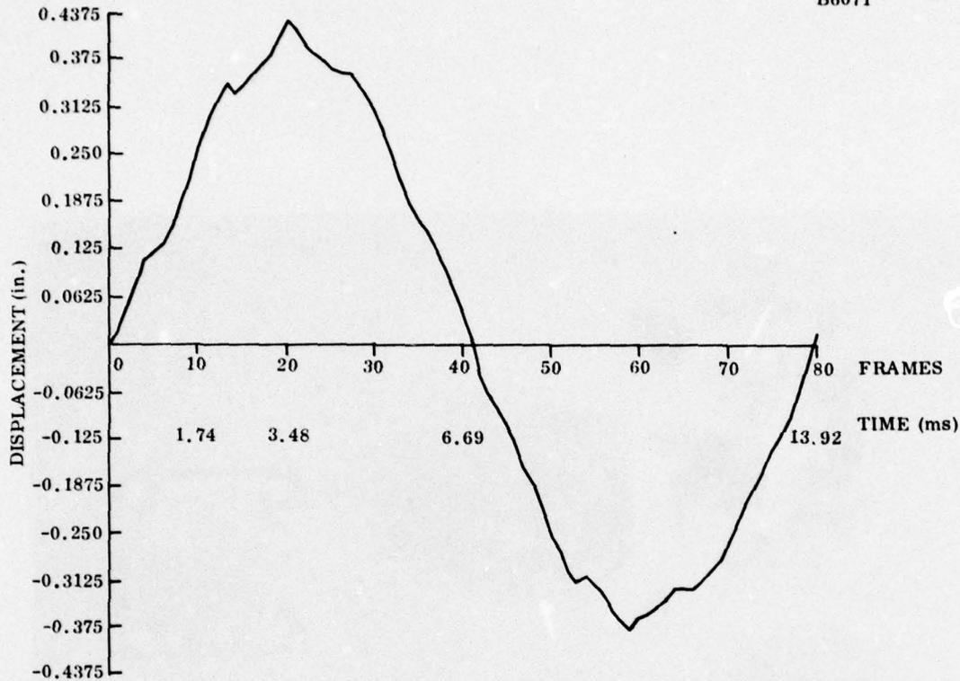
Figure 4-15. Beam Response to Impact with Indiana Sandstone Projectile (11 I. S.)
