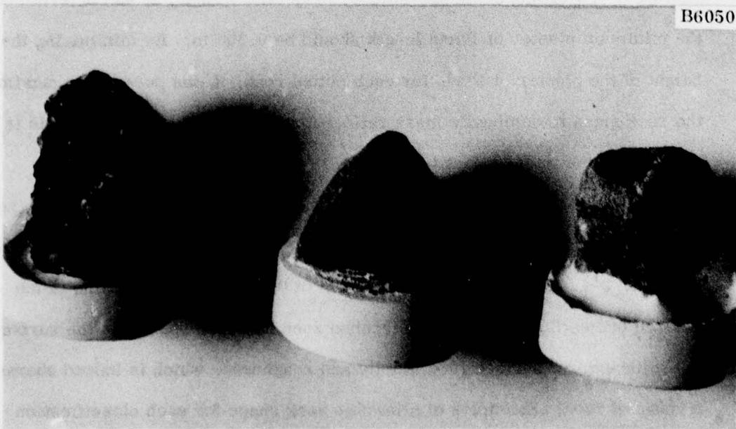
Figure 3-3. Projectiles Encapsulated in Plaster of Paris
