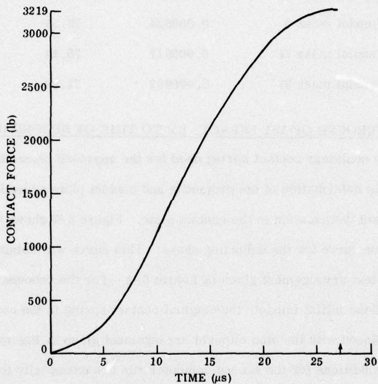
Figure 6-6. Contact Force vs Time During Impact Loading Phase
