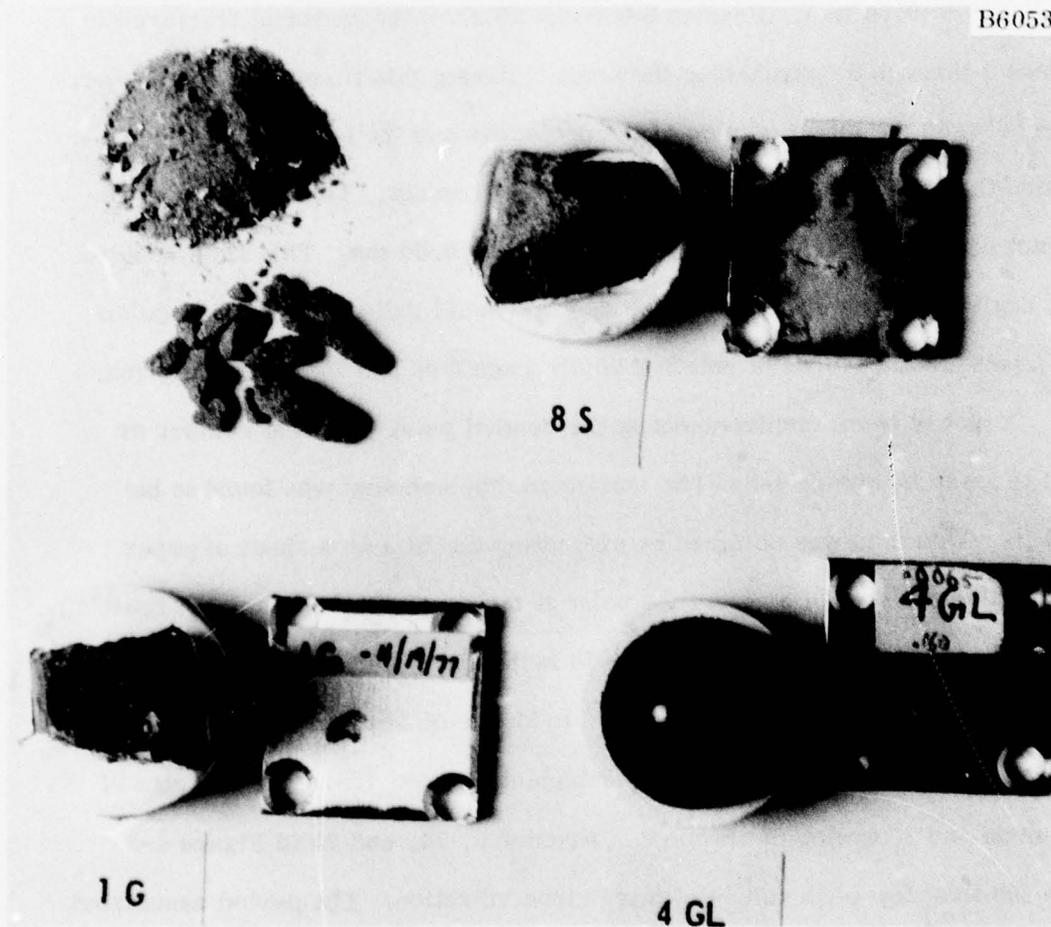
Figure 4-1. Projectiles and Associated Beam Contact Plates Following Impact (8S-Indiana Sandstone, 1G-Gabbro, 4GL-Glass Sphere)
