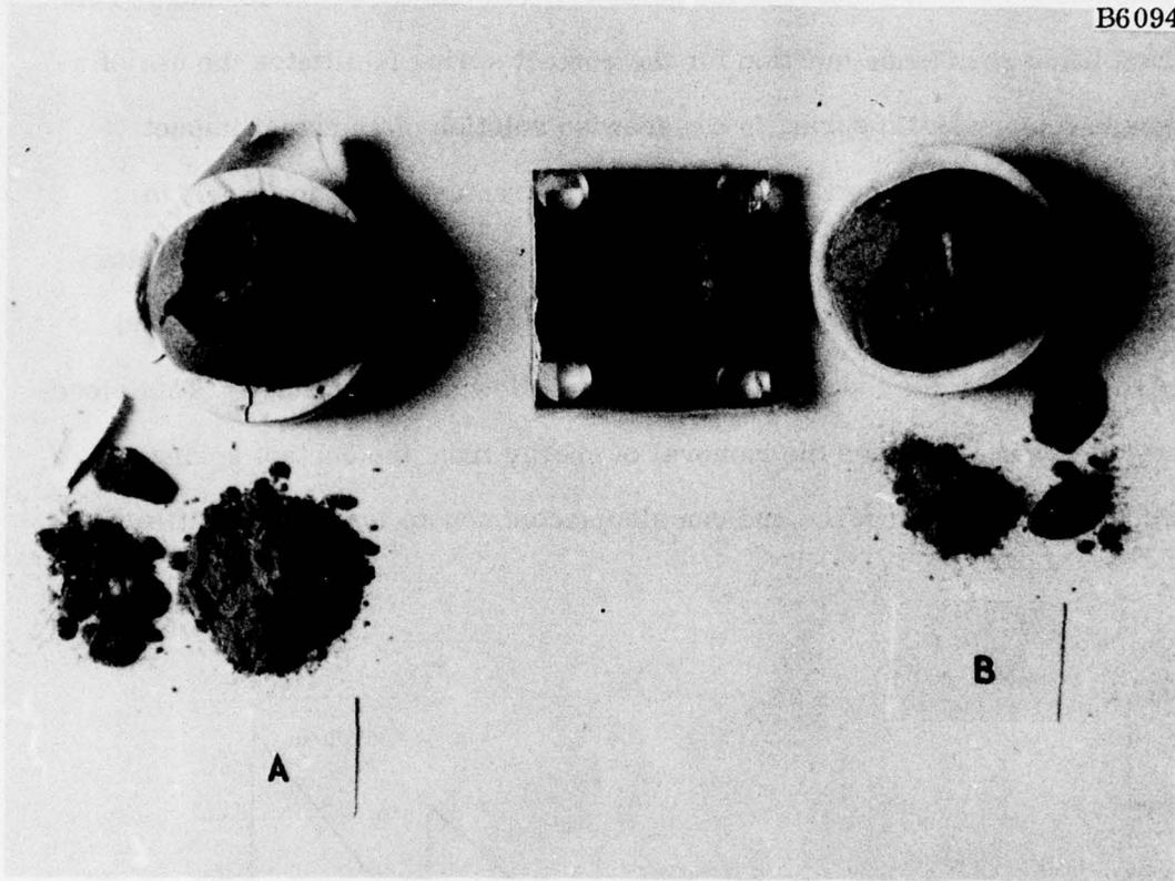
Figure 6-14. Indiana Sandstone Projectiles A and B Following Static Compression Against 6061T6 Aluminum Plate
