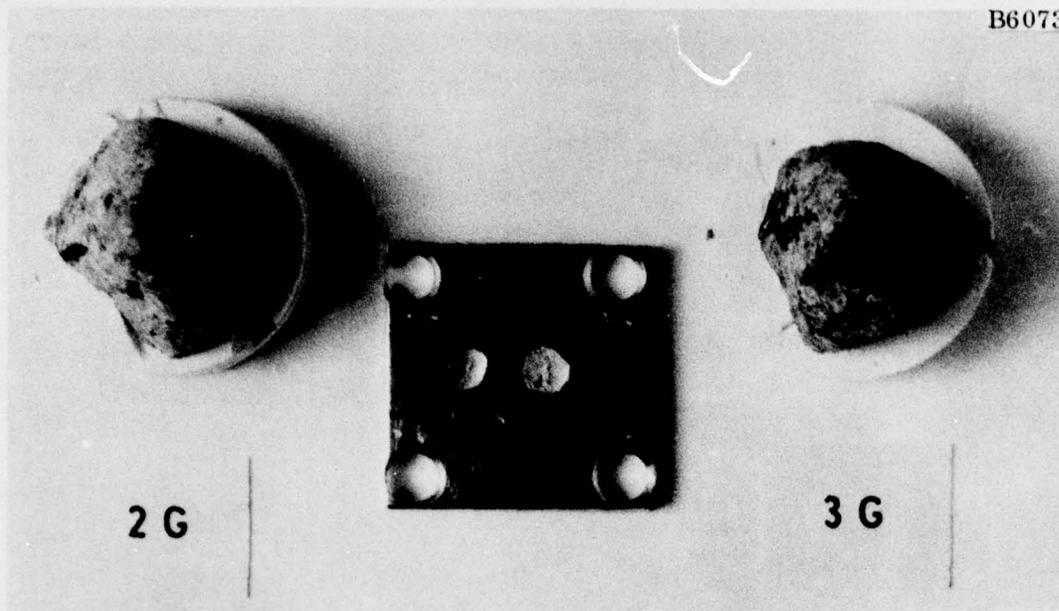
Figure 4-17. Intact Gabbro Projectiles and Indented Contact Plate
