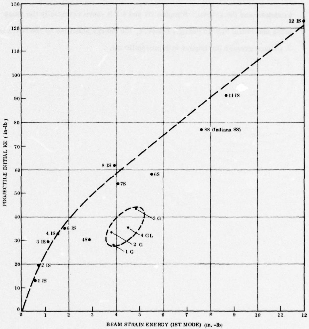
Figure 5-5. Projectile Initial Kinetic Energy vs First Mode, Beam Strain Energy
