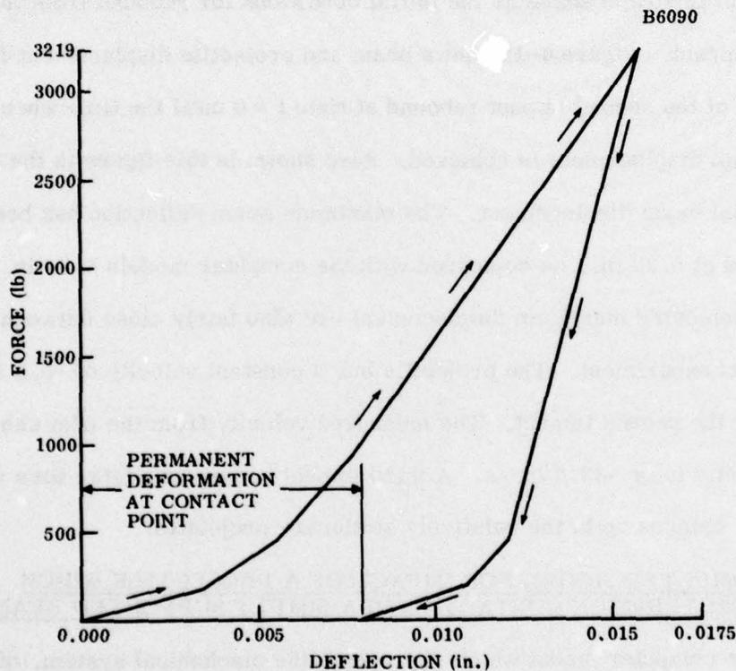
Figure 6-10. Contact Spring Force Deflection During Loading and Unloading Phase for Computer Model Initial Impact
