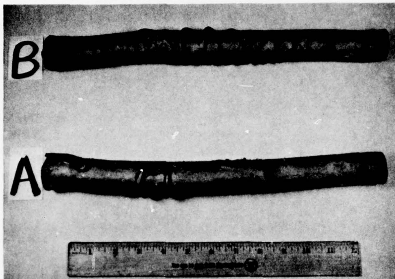
(a) Extrusions A6517 and B6518 - W-HfH 2 -C Material with Steel Clad in Place (Process A)
