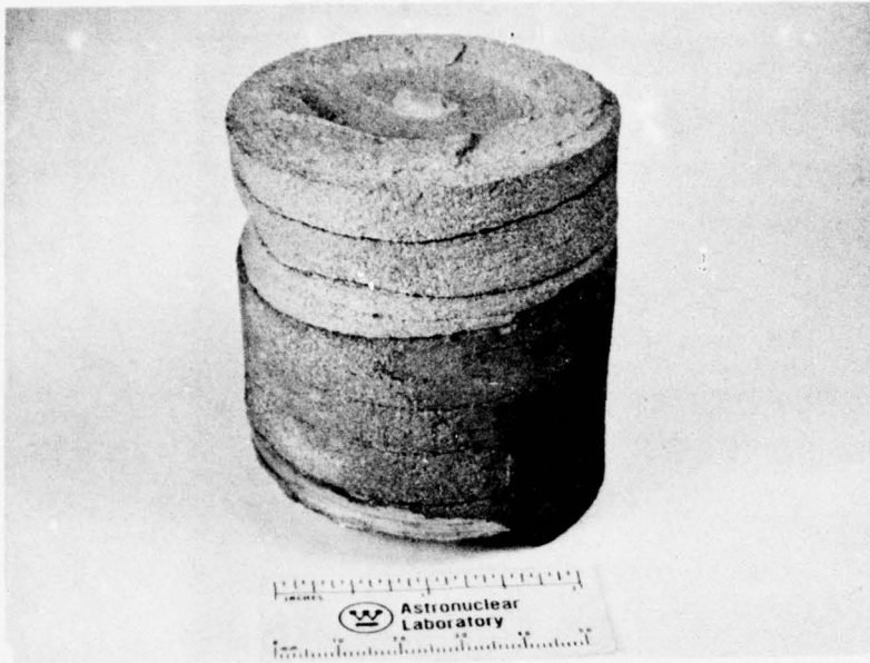
(a) Declad Hot Pressed WHfC Prealloyed Powder Compact
