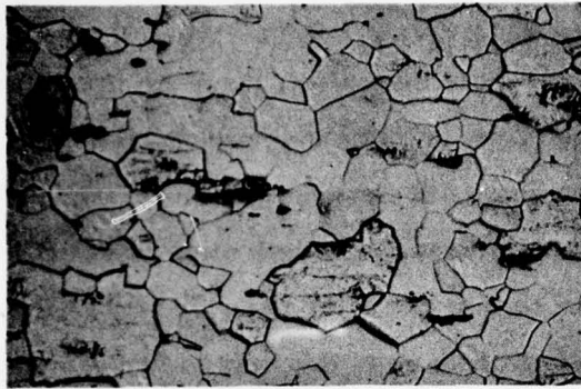
Solution Annealed 1/4 Hour/4600°F + 1 Hour/2500°F - Longitudinal
