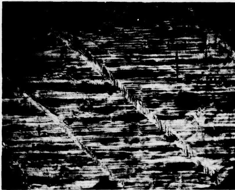
FIGURE 4 DOMAIN WALLS IN A TbFe 3 SINGLE CRYSTAL (100) FACE AS REVEALED BY FERROFLUID. APPLIED H \approx 1.2 \text{ kOe} AND IS UP IN THE PHOTO.
