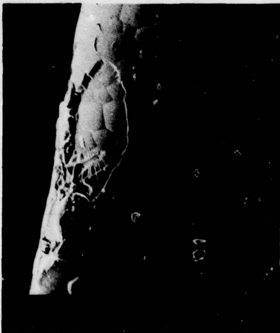
Figure 9. SEM of Boron fiber electrocoated by styrene-maleic anhydride copolymer.
