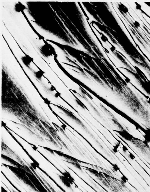
5. Photoemission micrograph of a cold-worked brass with 6% deformation. Note the  $\beta$ -grains in a deformed  $\alpha$ -structure. The deformation of the  $\alpha$ -matrix is evidenced by deformation twins. (L. Wegmann, Fifth International Congress on X-Ray Optics and Microanalysis, 9 September 1968)
