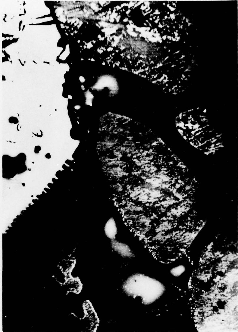
10B. This micrograph was taken at 1700°C and shows that the glass matrix has melted and begun to attack the alumina. (L. Wegmann, *Journal of Microscopy* 96, 1, 1972).
