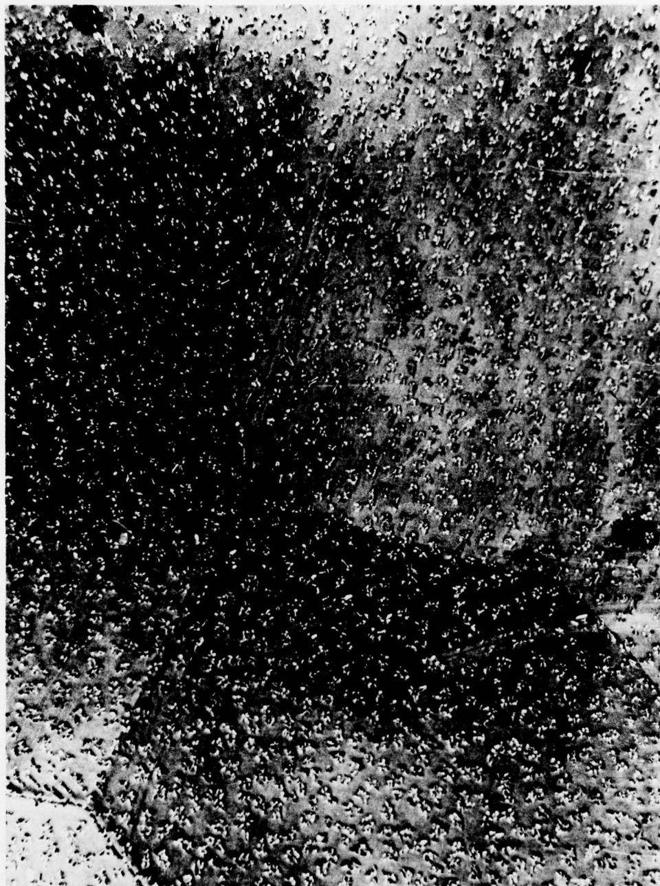
9. Photoemission micrograph of a nickel surface oxidized at 900°C *in situ* at an oxygen pressure of  $10^{-4}$  Torr. (L. Wegmann, *Journal of Microscopy* 96, 1, 1972).
