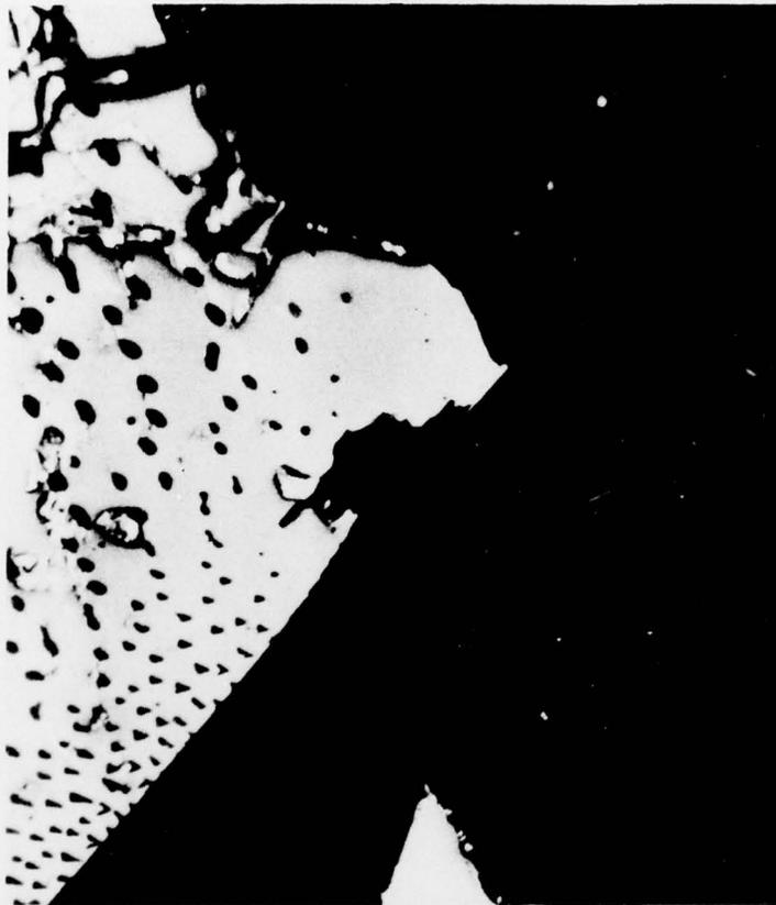
10A. Highly refractory brick consisting of  $ZrO_2$  (grey),  $Al_2O_3$  (white) and a glass matrix (black). Photoemission micrograph taken at  $700^\circ C$ .
