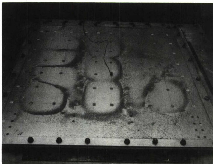
Figure 40 Bonded Panel Sand Pattern, 307 Hz
