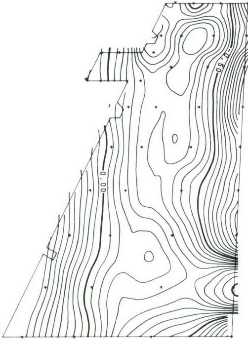
Figure 10 F-4 Rudder Mode Shape from Digital Impact Method, 28 Hz
