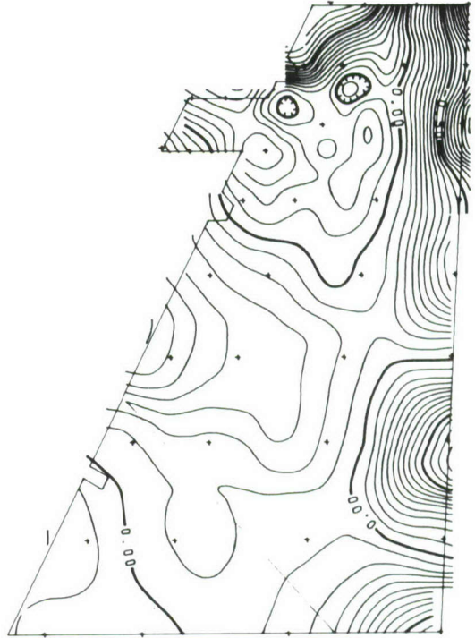
Figure 19 F-4 Rudder Mode Shape from Digital Impact Method, 396 Hz
