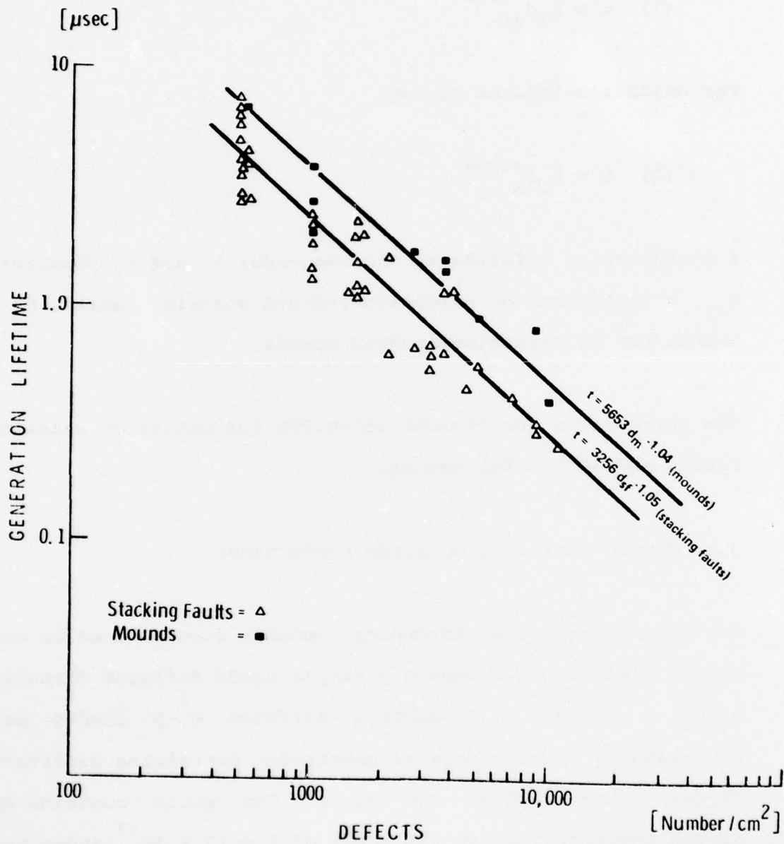
Fig. 27. Lifetime vs. defect dependency.
