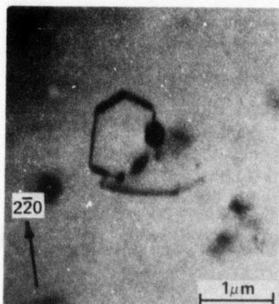
Fig. 15. Electron micrographs showing the shape of precipitate is hexagonal on (111) projection.
