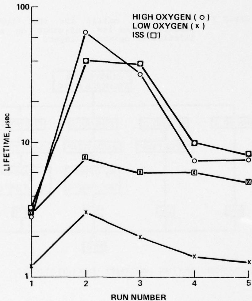
Fig. 21. The influence of various heat-treatments on the lifetime of epitaxial layers
