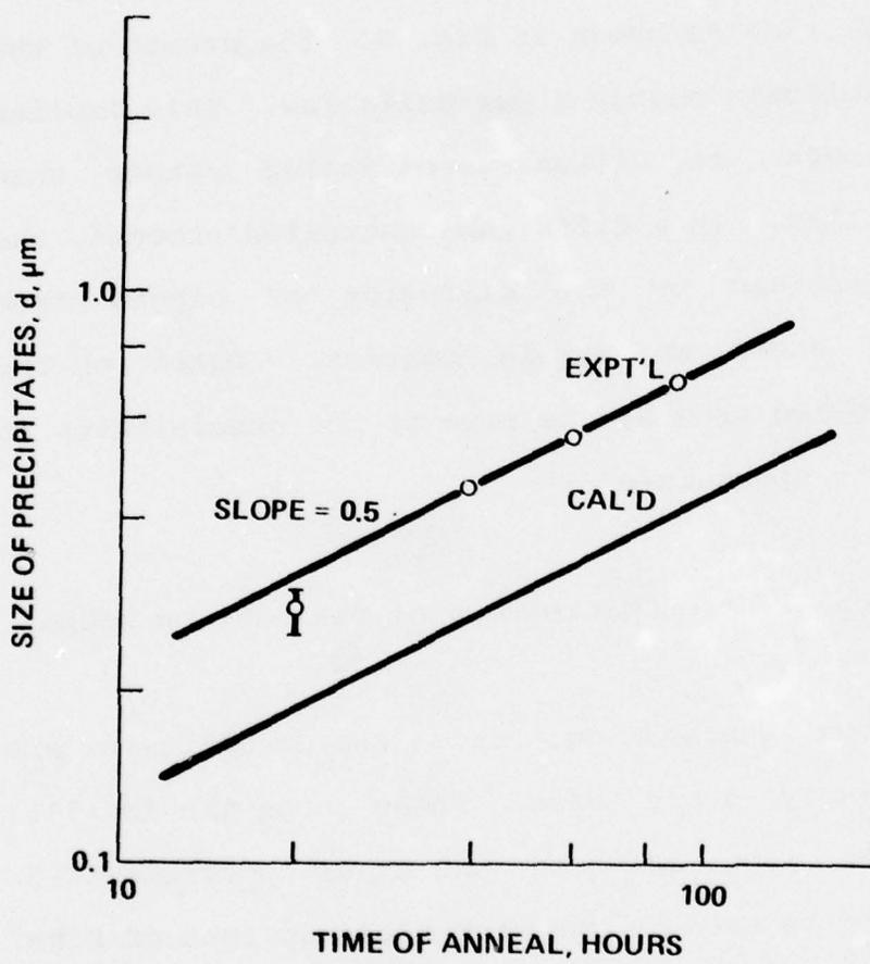
Fig. 9. The size of precipitates as a function of time of annealing at 1100°C
