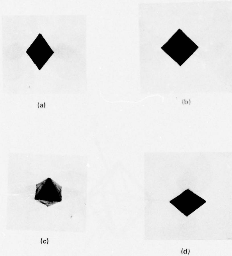
Fig. 8. A model of a precipitate on (a) (011), (b) (010), (c) (111), and (d) (101) projection.
