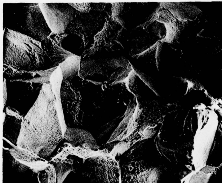
Figure 20. Heat Affected Zone Fracture Surface of Ti-8V-4Cr-2Mo-2Fe-3Al Alloy. Post Weld Aged at 1150°F (621°C) for Eight Hours. X160
