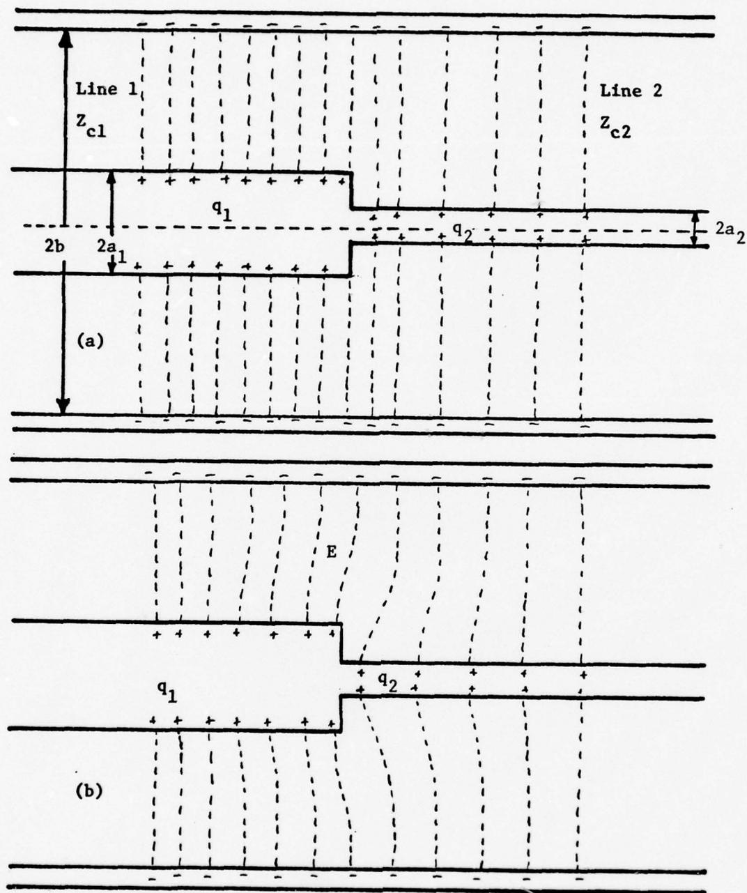
Fig. (2.4) (a) Zero order (b) Approximate Actual Distributions of Charge per unit length and Radial E field in Coaxial Line.
