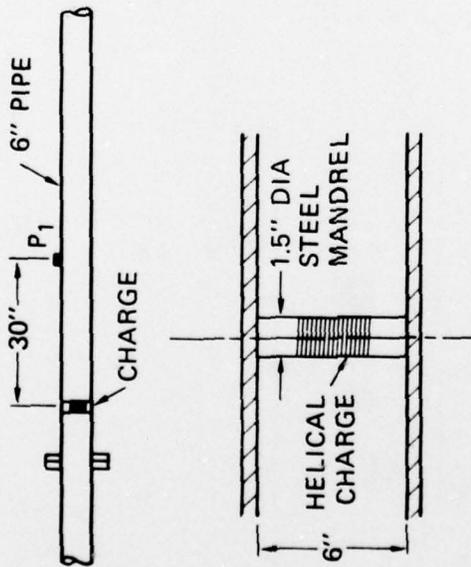
(a) CONFIGURATION OF VERTICAL HELICAL CHARGE
