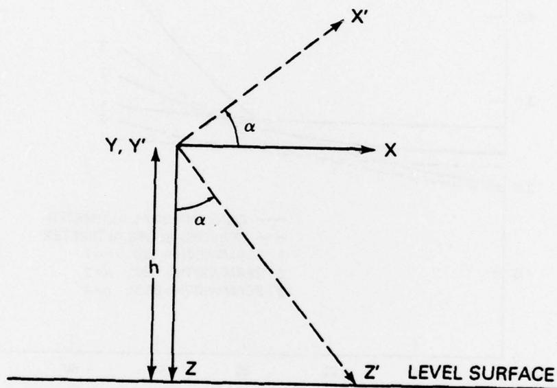
Fig. 9 - Coordinate system used for oblique incidence
