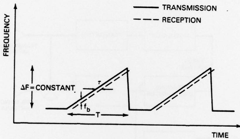
Fig. 3 - Asymmetrical modulation used in
