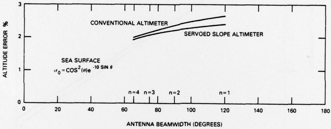
Fig. 8 - Altitude vs antenna beamwidth for two altimeters
