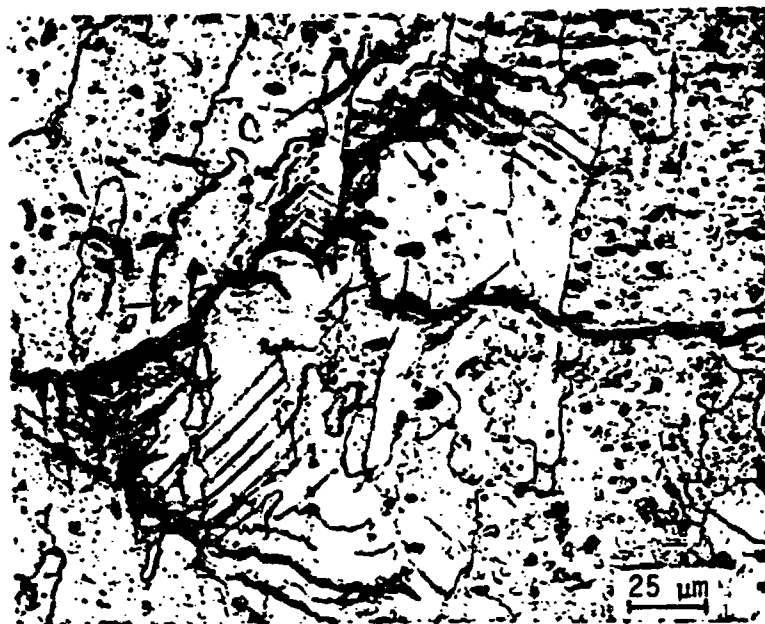
FIG. 9-Light micrograph illustrating crack path of an underaged (4 h at 120°C) Al-6Zn-2Mg-0.11Zr alloy. Compact tension sample, laboratory air, \Delta K = 10 \text{ MPm}^{-\frac{1}{2}} . Keller's etch.
