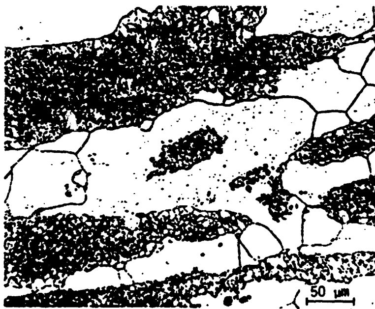
FIG. 2-Light micrograph illustrating mixed recrystallized (light) and unrecrystallized (dark) structure of commercially processed 7050-T6X1 plate. Etched in 25% \text{HNO}_3 for 3 min. at 70°C.
