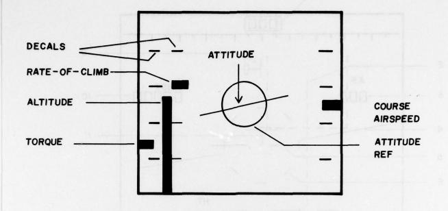
Figure 2. Avionics Laboratory enroute flight display symbology (20).
