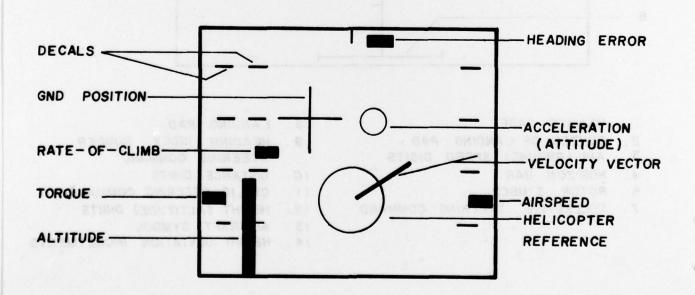
Figure 3. Avionics Laboratory hover display symbology (20).
