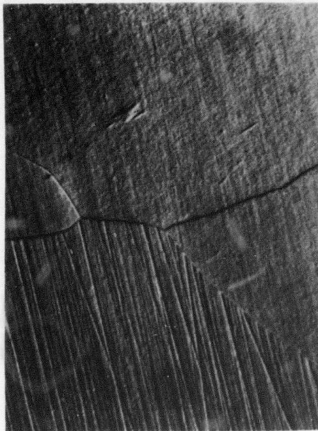
Figure 6. Etching anisotropy in \text{CaF}_2 .
