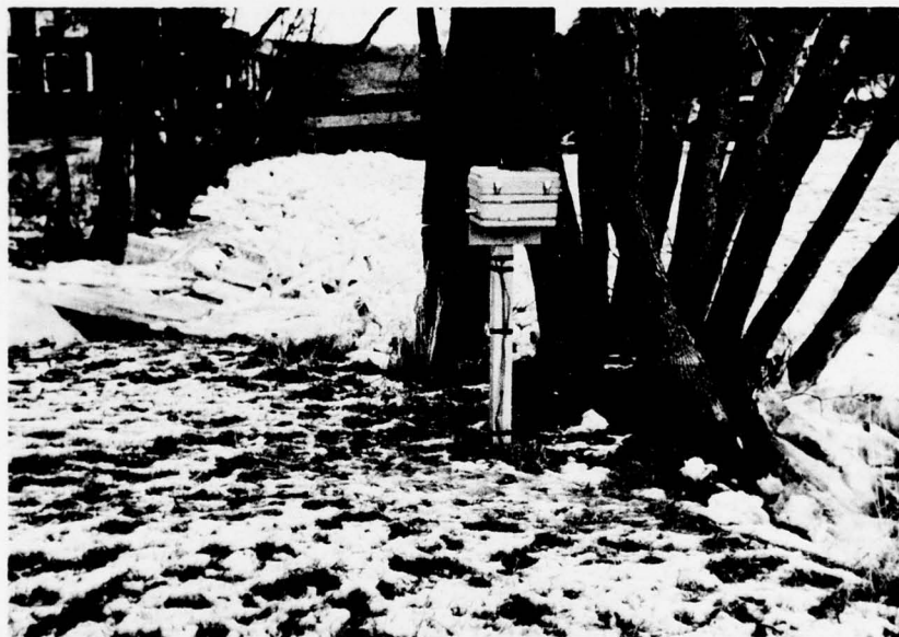
Figure 2. Stage recorder installation.
