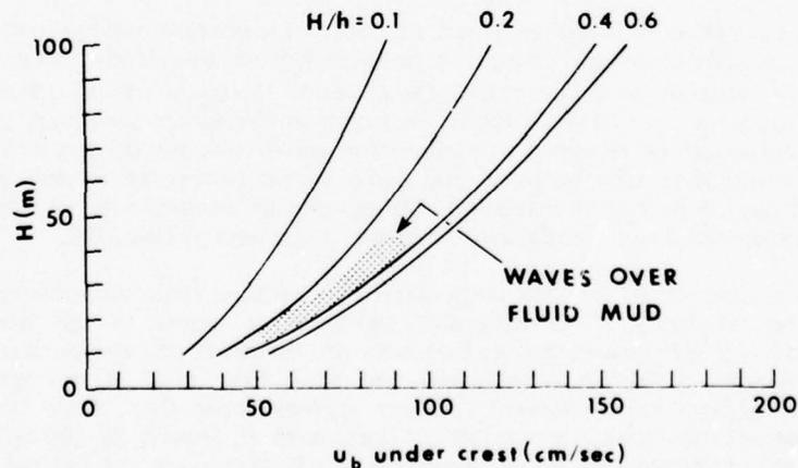
Figure 21. Theoretical bottom particle velocities under solitary wave crests.
