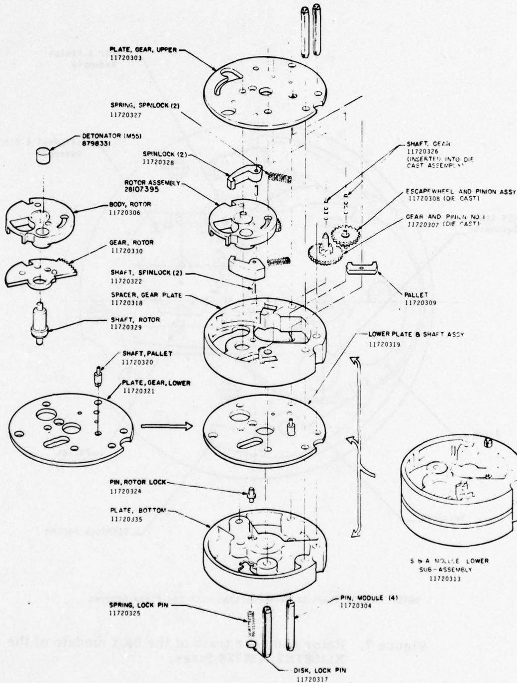
Figure 8. Exploded view of the XM587E2/XM724 fuze S&A module.
