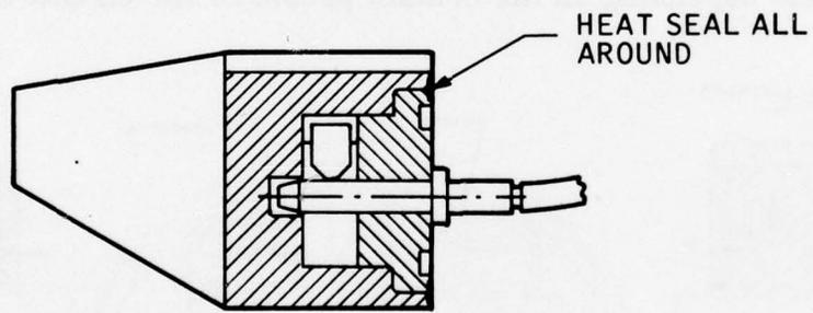
Figure 22. Spin switch initial design layout.
