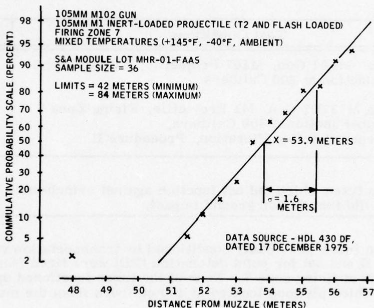
Figure 20. Results from fire on mechanical arming test.
