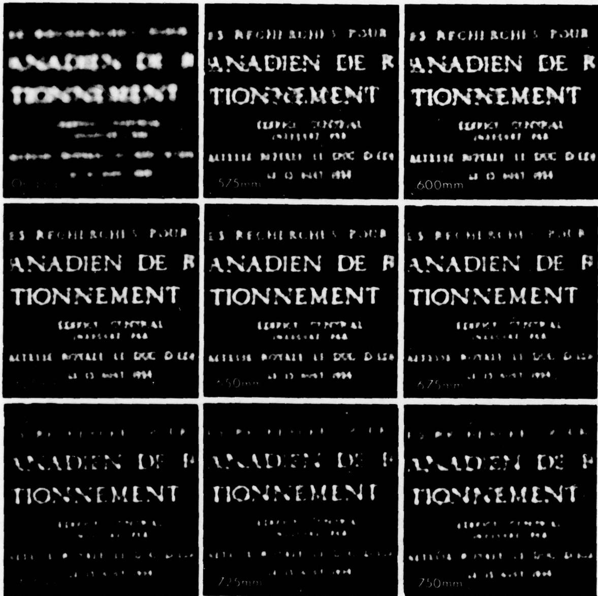
FIGURE 16 Determination of the OTF of the blur interactively. A region of a blurred photograph is shown in the upper left. Assuming the blur is due to an out-of-focus camera, the image was restored using 8 different assumed values of blur-circle diameter. These values, which are written in the lower left of each image, varied in  $0.025$  mm steps from  $0.575$  mm to  $0.750$  mm. The restoration is clearly optimum for a blur-circle diameter of  $0.675$  mm.
