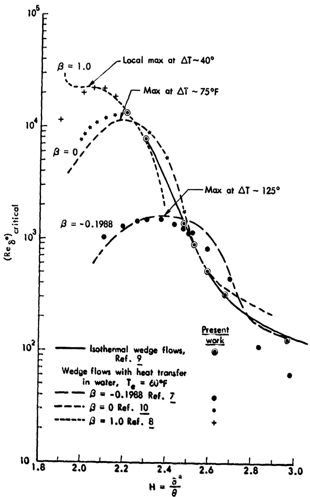
Fig. 1—Comparison between modified Dunn-Lin method and numerical solution of the Orr-Sommerfeld equation
