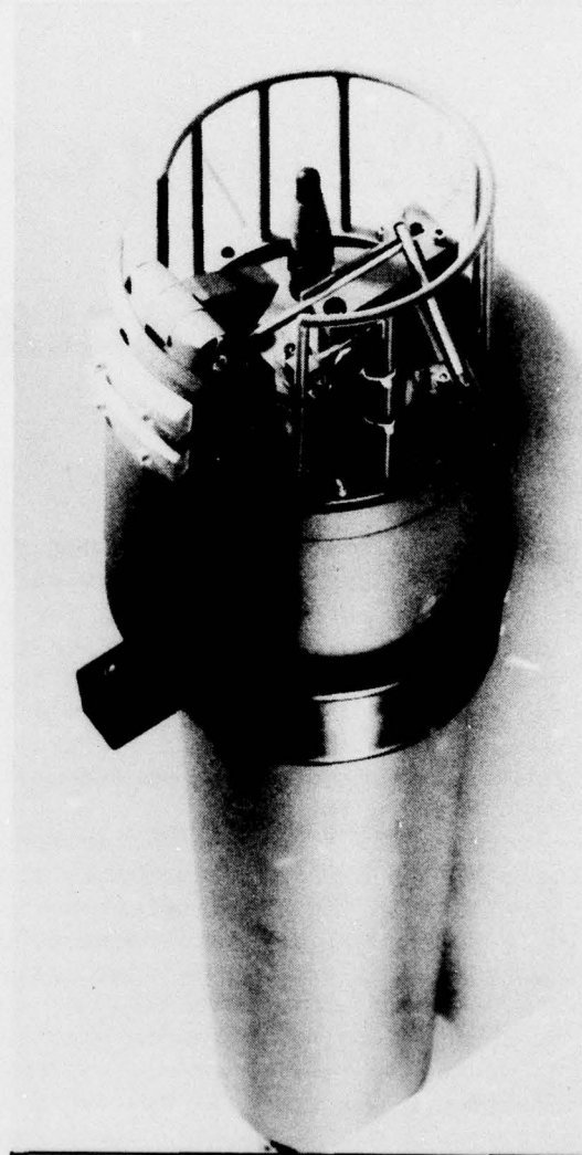
THE VANE HELD IN PLACE BY THE PRESSURE RELEASE PIN
