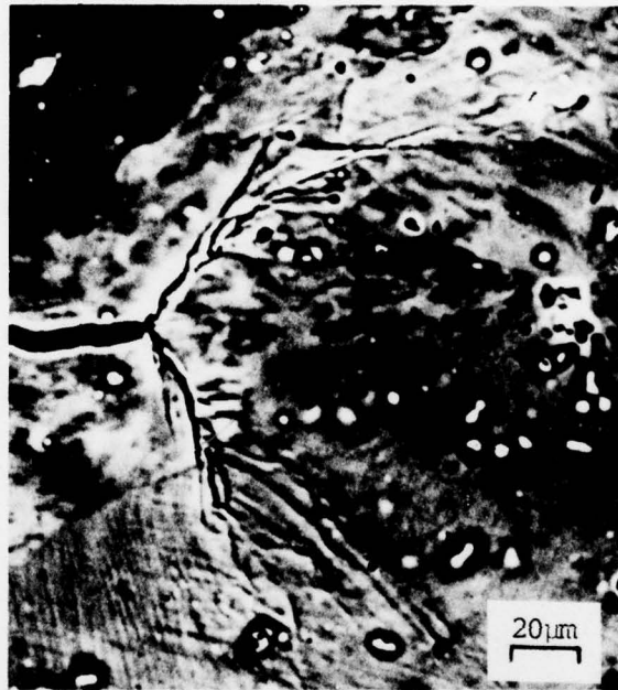
Figure 5. Subcell formation in the vicinity of a fatigue crack tip subjected to a one cycle overload of K = 26\text{MN/m}^{3/2} as observed by channeling contrast. 7075-T6 Aluminum Alloy, 20 keV
