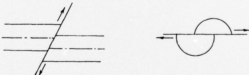
In the Phase I study, interactions of the type shown in Figure 1 between deeply-buried tunnels and *in situ* joints in granite when loaded by 1 kb stress waves were investigated using both analytical models and two-dimensional finite
