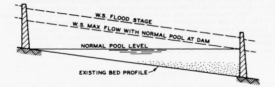
pool level at the dam, open river conditions prevail and the gates are in the raised position (fig. 1). With this condition the water-surface slope
