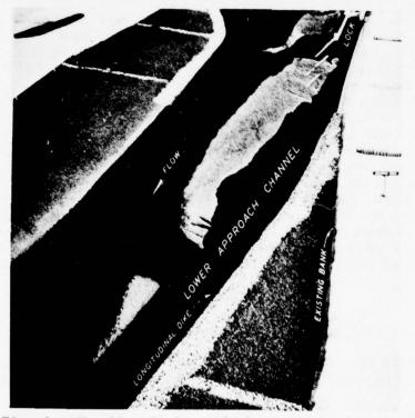
Fig. 3. Shoaling in lower lock approach with three wing dikes at end of lower guard wall
