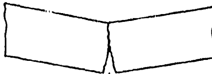
Figure 2B. Typical Flexural Failure
