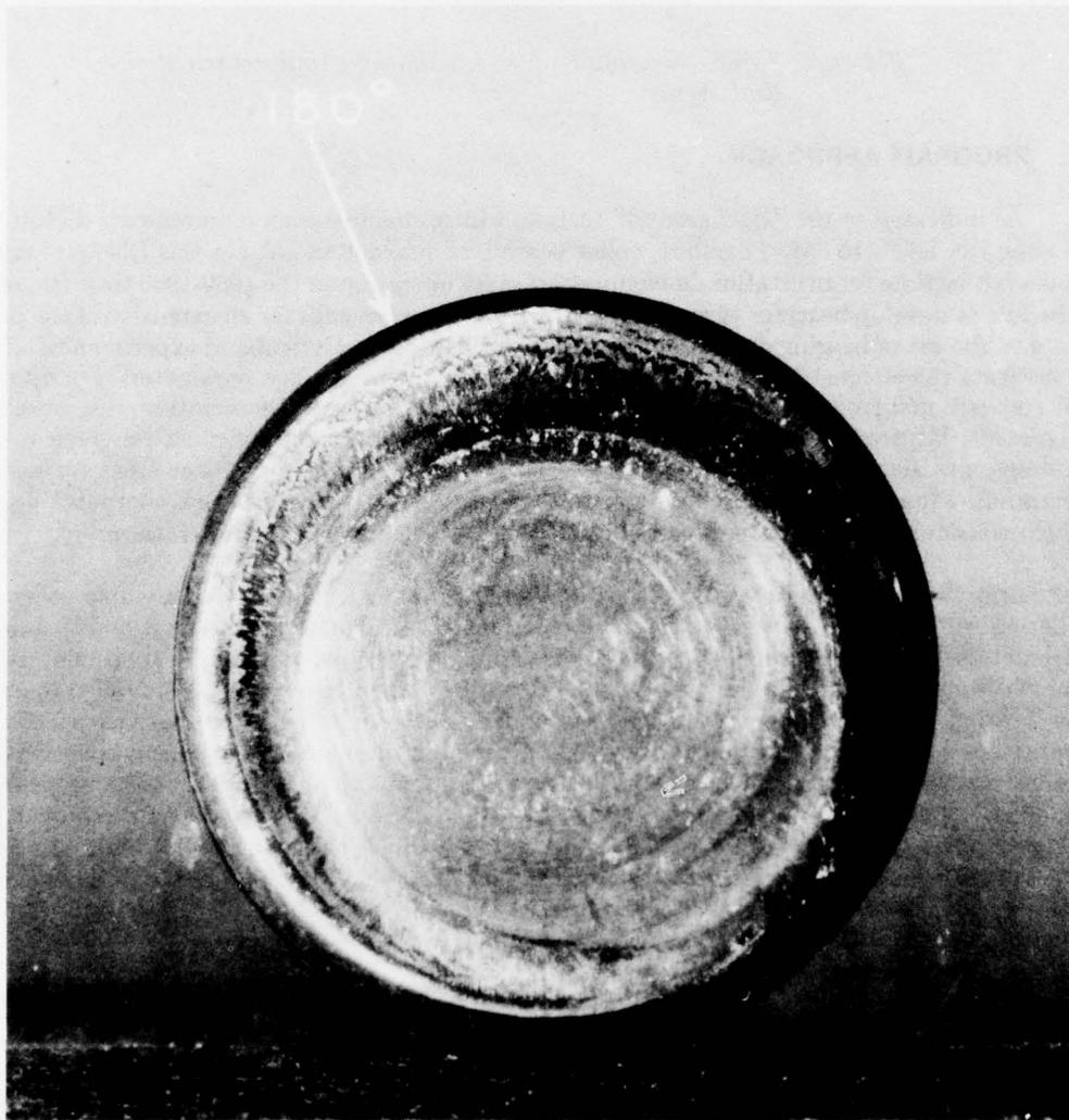
*Figure 1. Eccentric Roller End Wear*
