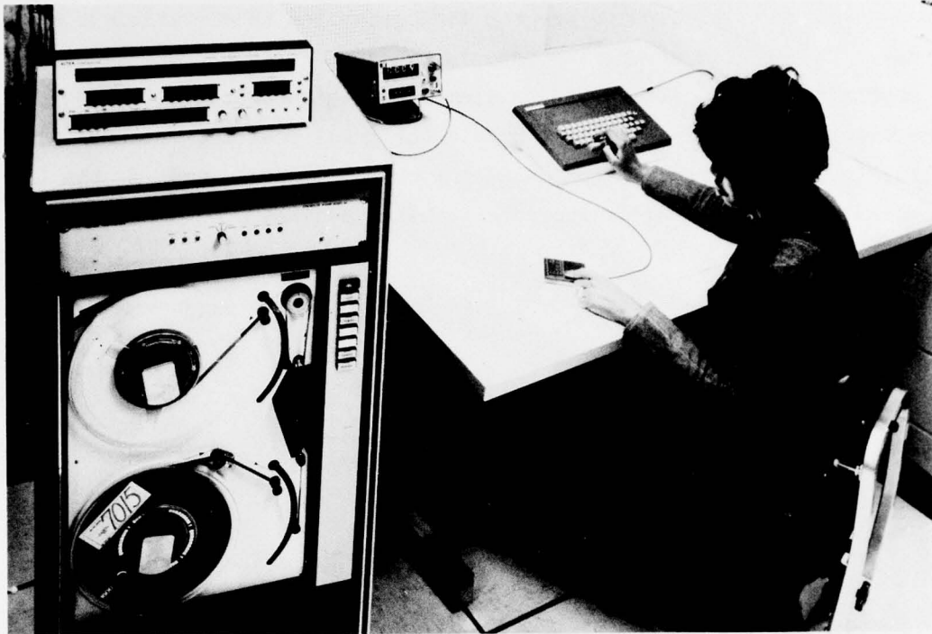
Figure C2. Technician transforming contour lines from topographic map into digitized data
