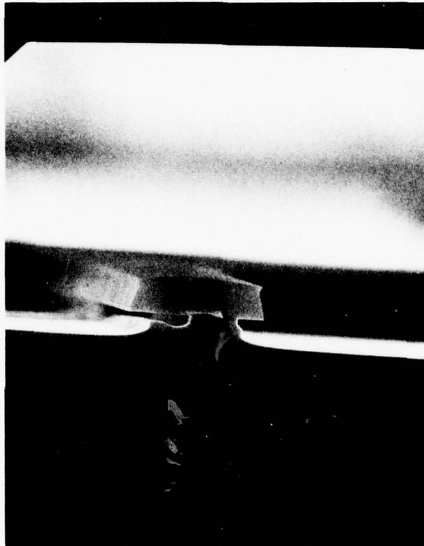
Fig. 16. SEM photomicrograph of a gate cross section during the early stages of the GaAs etching process in the presence of a 2-micron wide AuMg stripe (bright area embedded in the photoresist). The top 7-micron wide stripe is a AZ1350J photoresist pattern. Undercutting towards the metal is intolerably high.
