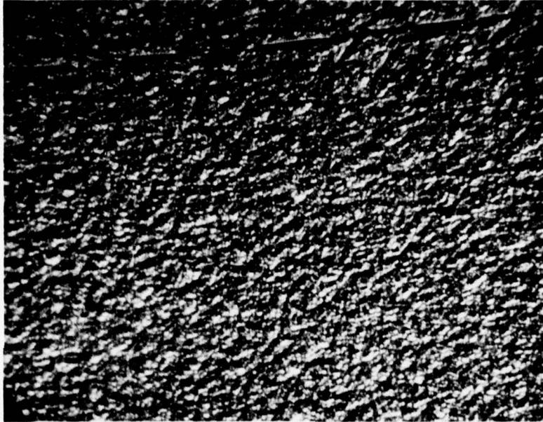
Fig. 8. Nomarski contrast photomicrograph of the n-type GaAs active layer after the  $\text{Al}_{0.5}\text{Ga}_{0.5}\text{As}$  having an acceptor concentration of  $2 \times 10^{18} \text{cm}^{-3}$  has been removed by selectively etching. The magnification is 1400.
