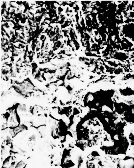
(a) Fatigue - SCC area at end of precrack.
