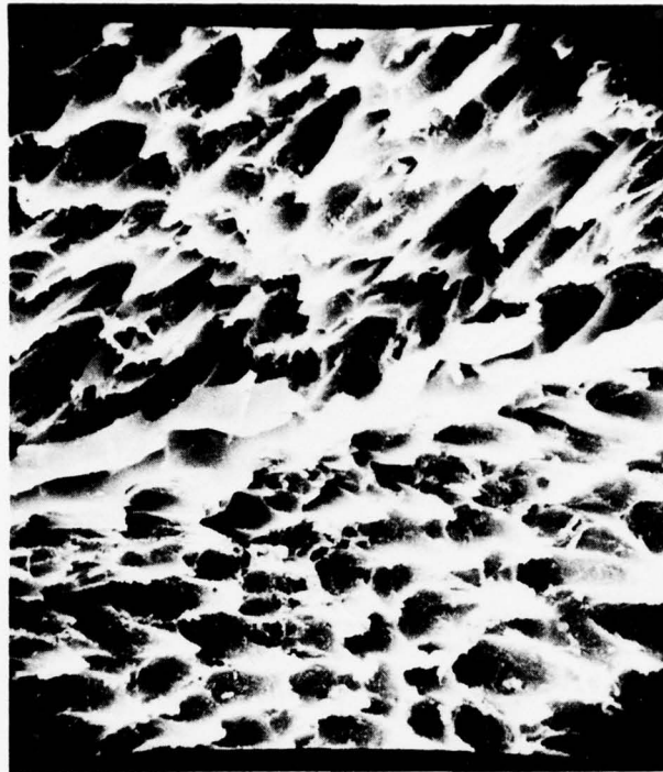
(a) NRL SAMPLE SHOWING INTERLAMINA REGION AFTER ETCHING (X1000).
