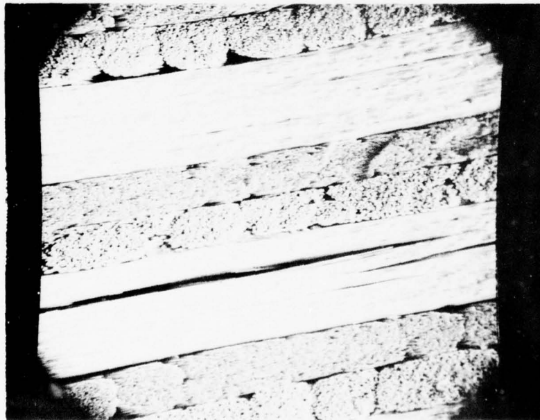
(b) NSRDC SAMPLE SHOWING FIBER LENGTHWISE AND ON EDGE AFTER ETCHING (X50).
