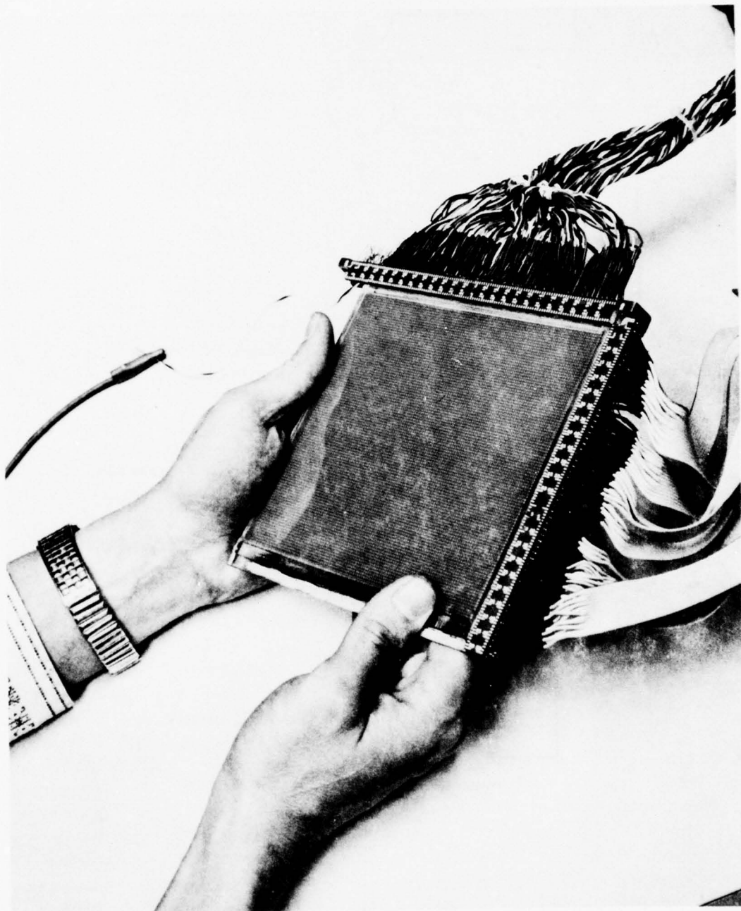
Fig (28) Completed, sealed display
