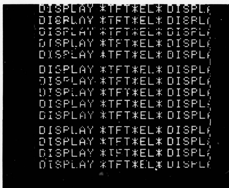
Fig (30) Operational 6" x 6" 30 lpi displays (2-level)
