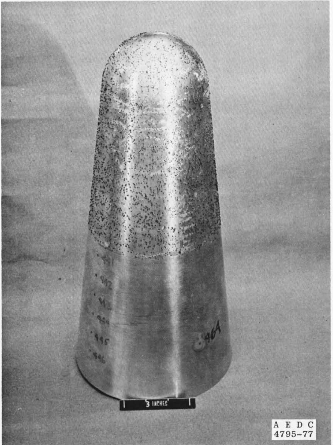
c. Blunt nose, r_n = 2.187 in., 25-mil grit Figure 7. Concluded.
