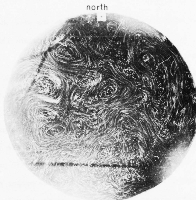
3-16 (a) 2D turbulence in the sliced cylinder model: the steadily forced case. Laboratory parameter values are \Omega = 5.1 rad/s, \omega = 0.43 rad/s, H = 25 cm, \alpha = 0.23 , w = 0.12 cm/s.
