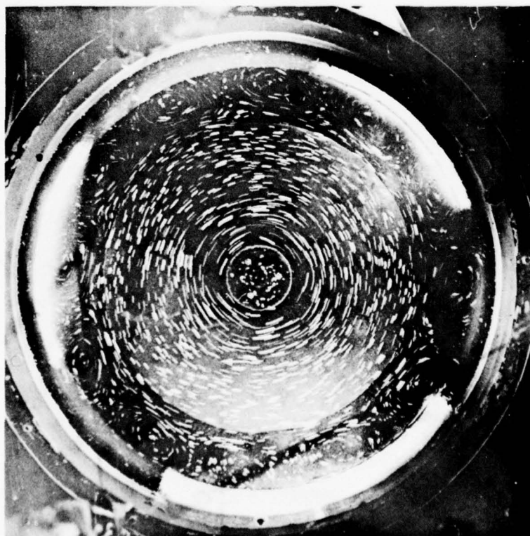
4-18 (a) The mean flow used in the critical layer experiments (b) The steady state of run 1.
