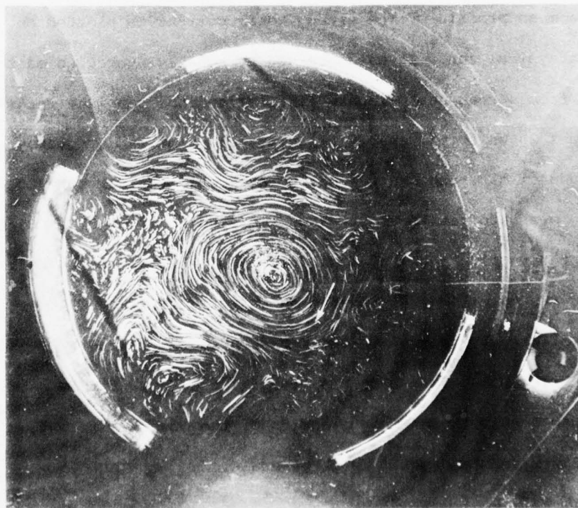
3-8 Turbulent flow on a polar \beta -plane. Experimental parameter values are U = 3.92 rad/s, \omega = 0.4 rad/s, H = 14.5 cm, w = 0.12 cm/s
