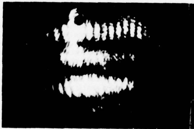
Figure 12. Resolution of a 2-mm bar pattern on the TV monitor. The 2-mm horizontal bar pattern in the test object shown in Figure 11 was insonified at 3 MHz with acoustic magnification of 3.6 in the surface holograms. Three of the 2-mm openings are shown here with a superimposed diffraction pattern due to the irregularities.
