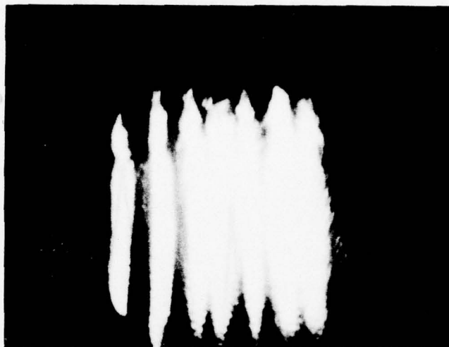
(a) OUTPUT PATTERN FOR HORIZONTAL 2-mm BARS WITH ACOUSTIC MAGNIFICATION OF 1:1 AT 3 MHz
