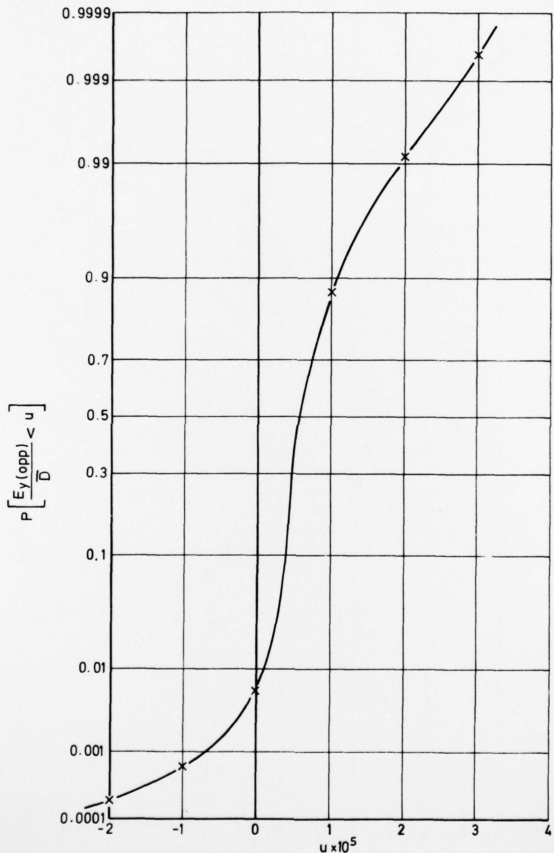
Fig 12 Distribution function assigned to opposite-direction lateral occupancy
