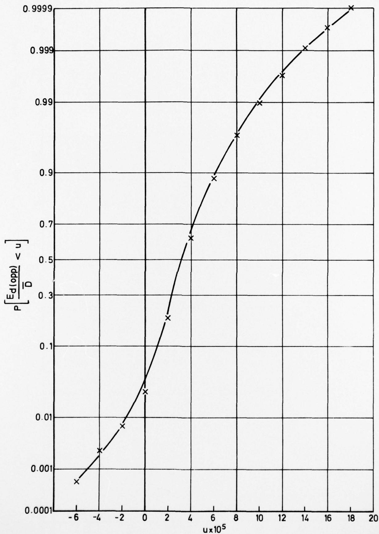
Fig 13 Distribution function assigned to opposite-direction diagonal occupancy
