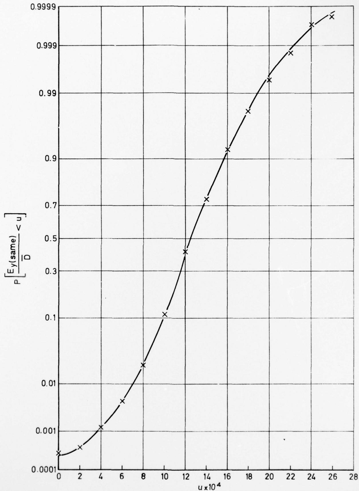
Fig 9 Distribution function assigned to same-direction lateral occupancy
