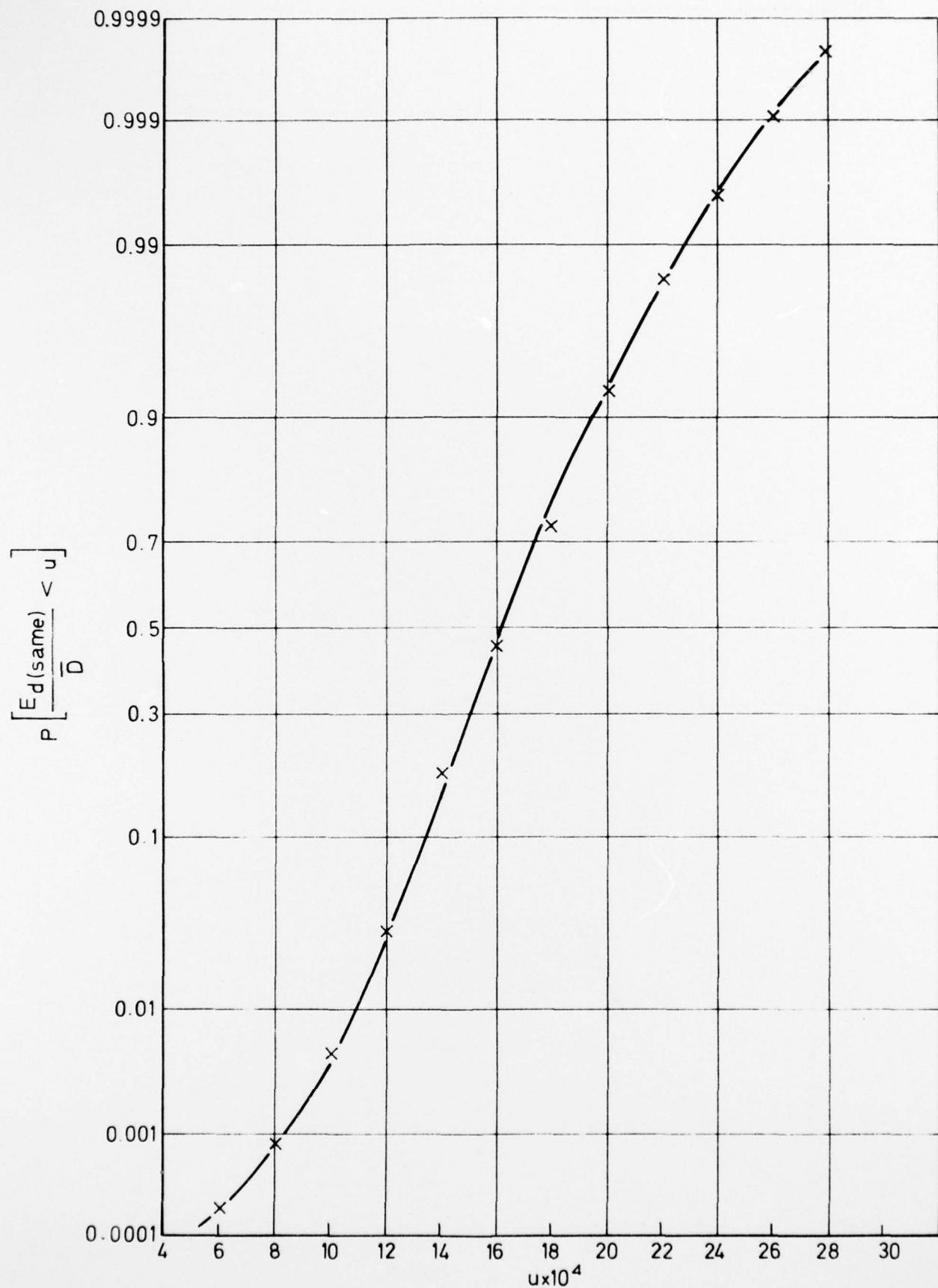
Fig 10 Distribution function assigned to same-direction diagonal occupancy
