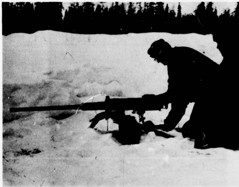
Figure 14. .50 caliber machine gun positioned to fire at snow trench.
