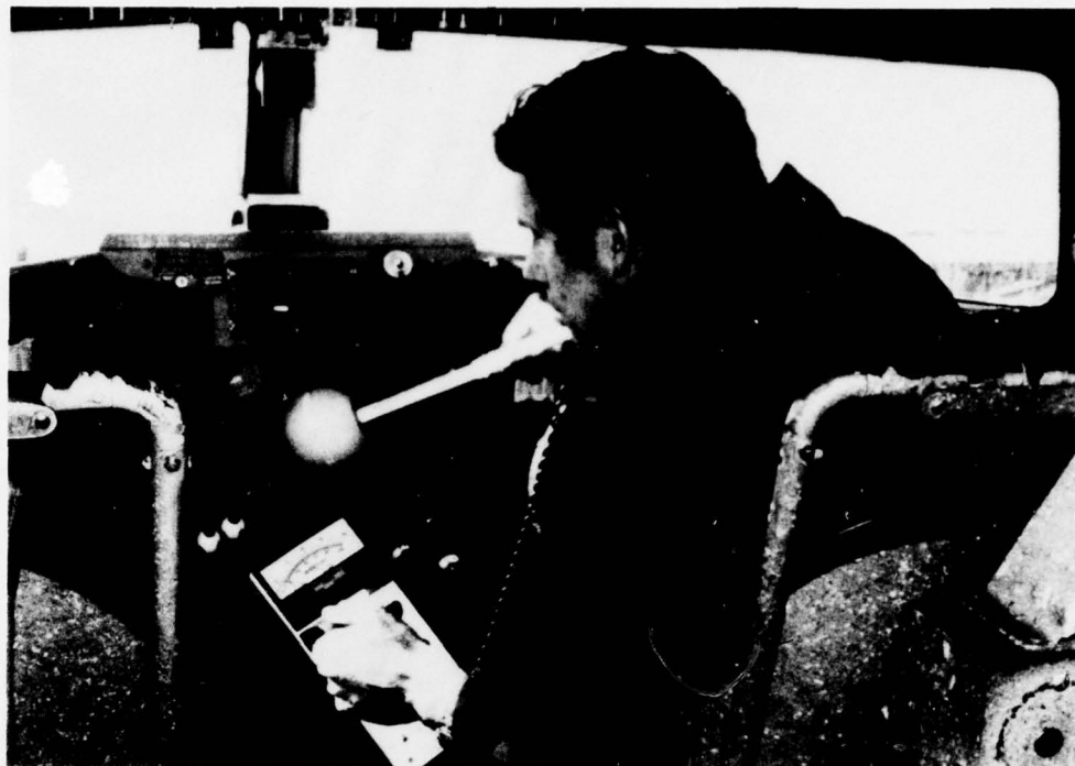
Figure 3-3. Photograph of an operator measuring stray fields with a CIM-1 radiation monitor in the cockpit of a DC-3 airplane.
