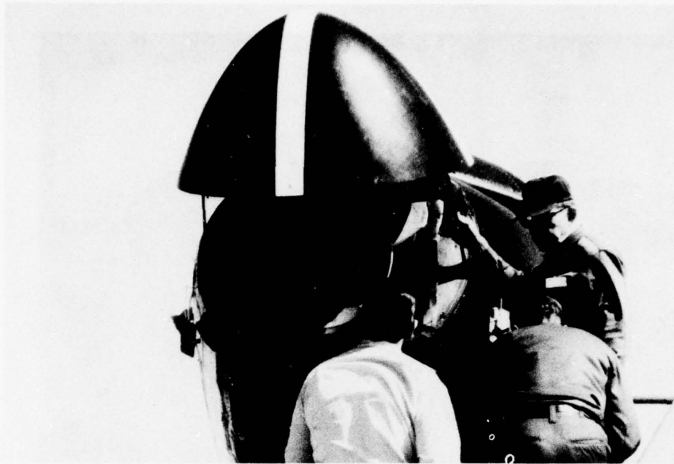
Figure 3-1. Photograph of airplane mechanics and a radar technician raising the radome of an RDR-1B radar antenna mounted in the nose of a DC-3 aircraft.
