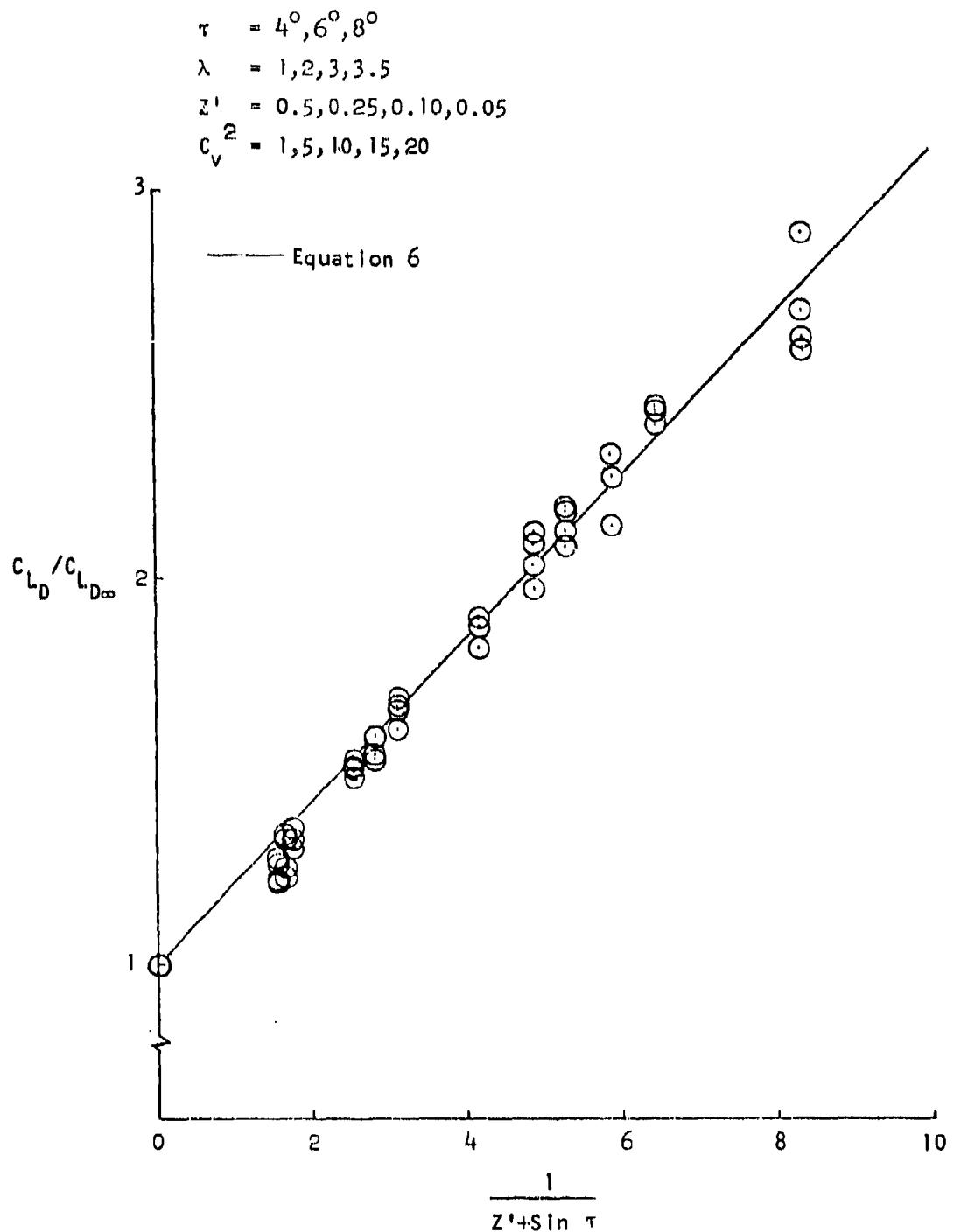
FIGURE 4. LIFT RATIO VERSUS RECIPROCAL DEPTH
