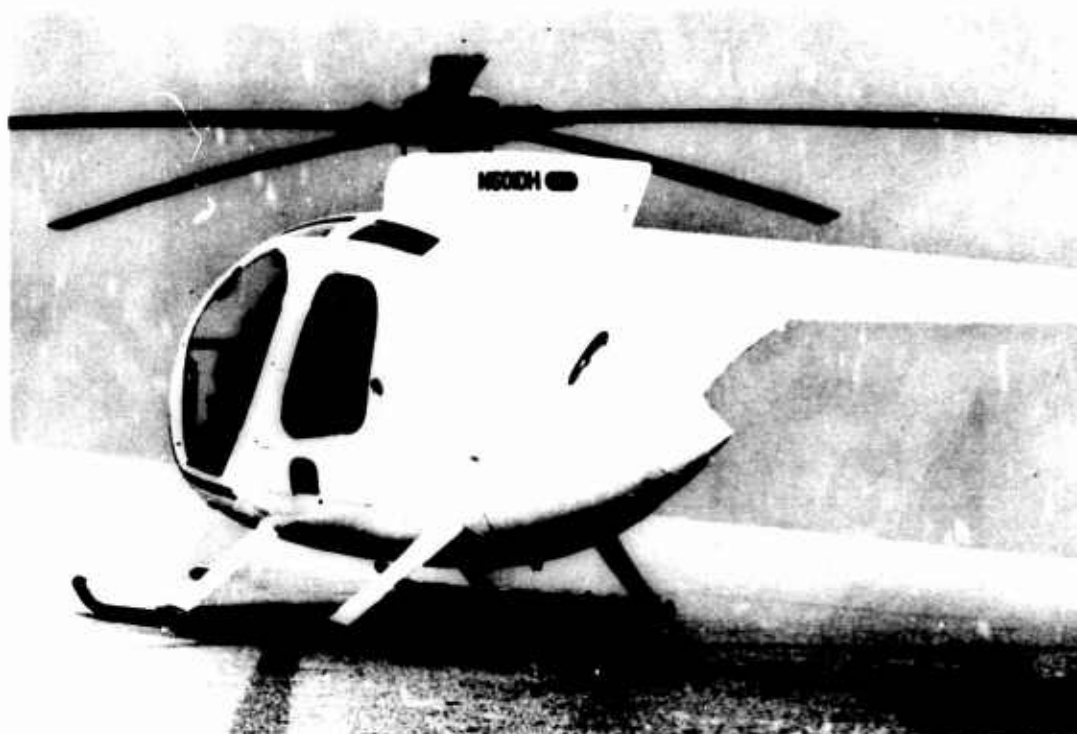
Figure 27. 500M-D With Exhaust IR Suppression
