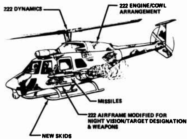
Figure 31. Model 222 Dynamics and Modified Airframe for Missiles.
